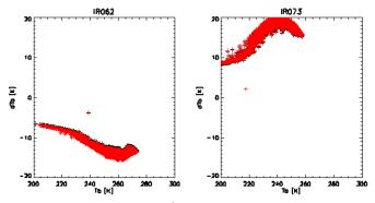
**Figure 2:** Spectral mismatches,  $\delta L_r$ , shown as brightness temperature differences [K] between water vapour channels of Meteosat-8 (black) and -9 (red) and Common Reference Channels.
