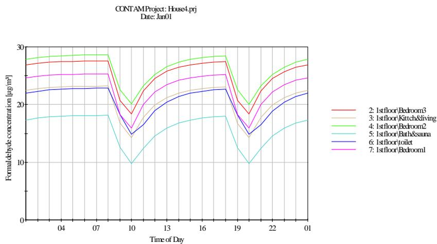
**Figure 4** The formaldehyde concentration when the SER from surfaces is  $10 \mu\text{g}/\text{m}^2\text{h}$ .
