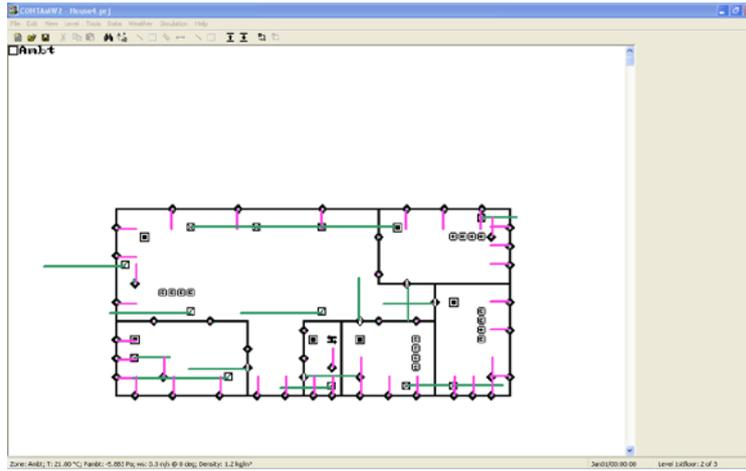
**Figure 2** Airflow simulation result for the model (air flows = green lines, pressure drop = red lines).
