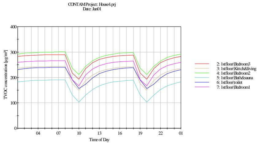
**Figure 3** The TVOC concentration when the SER from surfaces is  $92 \mu\text{g}/\text{m}^2\text{h}$ .
