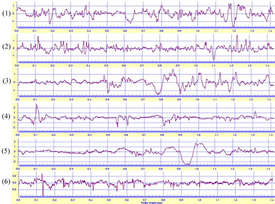
Figure 1. The virtual bullet signature standard consists of six digitized bullet profile signatures measured by a stylus instrument on six master bullets fired at the ATF and FBI. The virtual standard profiles shown above are modified profiles after curvature removal and Gaussian filtering defined in national and international standards [9,10] with a short wavelength cutoff of 0.0025 mm and a long wavelength cutoff of 0.25 mm. The vertical scale is in \mu\text{m} ; the horizontal scale is in mm.
