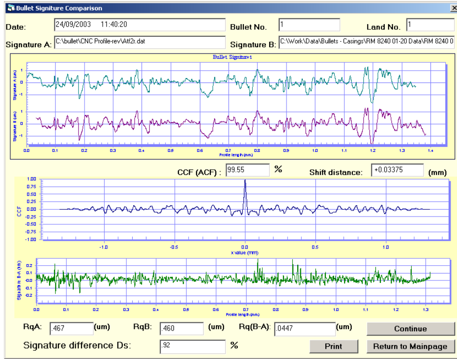
Figure 3. User screen for a bullet profile signature correlation of S/N SRM 2460-001 Standard Bullet (Signature B, shown as the second profile from the top) and the virtual standard (Signature A, shown on the top). The bottom profile shows the signature difference (B – A); the cross correlation function maximum CCF_{\max} = 99.55 \% \pm 0.12 \% ( k = 2 ), the signature difference D_s = 0.92 \% \pm 0.26 \% ( k = 2 ).
