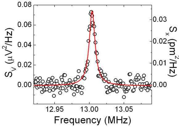
FIG. 3. (Color online) Thermal noise peak of NW (no drive) at 400 K. The axis on the left is the power spectral density of NW (minus amplifier background). The axis on the right is the conversion to picometers through the equipartition theorem. The peak rides on a frequency-independent amplifier background of  $5.2 \times 10^{-12}$  V<sup>2</sup>/Hz. The resonance frequency is  $13.0042 \pm 0.0002$  MHz with a width of  $10\,200 \pm 600$  Hz, for a mechanical  $Q = 1270 \pm 70$ .
