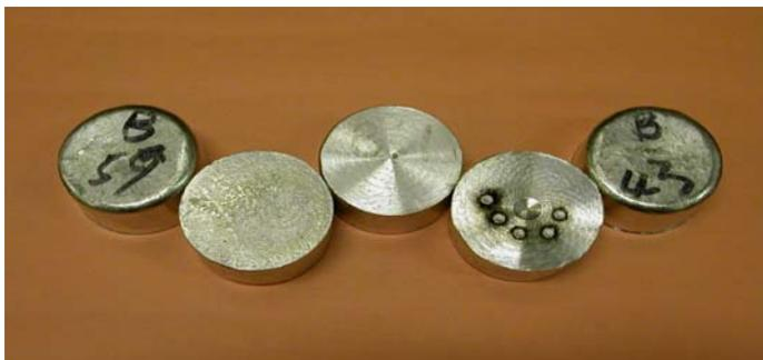
Semi-chill cast disks of SRM 1728 showing various stages in manufacturing and testing.
