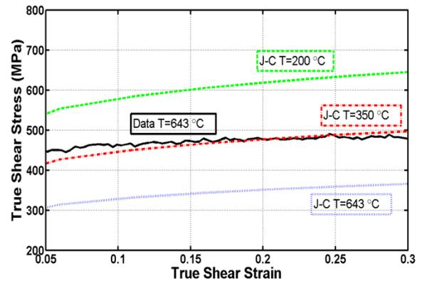
Figure 3: Data (solid curve) from pulse-heated compression test of an AISI 1045 steel sample that had been preheated to 643 °C, and then plastically deformed at a true strain rate of 3600 s<sup>-1</sup> (solid curve), and corresponding values of the Johnson-Cook model for AISI 1045 of Jaspers and Dautzenberg, with  $m=1$ , at three different temperatures, as indicated.
