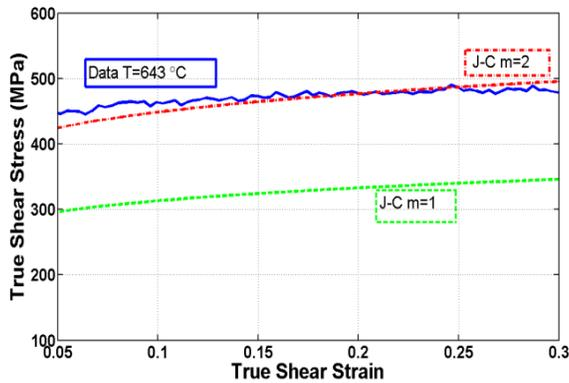
Figure 2; Data (solid curve) from pulse-heated compression test of an AISI 1045 steel sample that had been preheated to 643 °C, and then plastically deformed at a true strain rate of 3600 s<sup>-1</sup>, and corresponding values of the Johnson-Cook model for AISI 1045 of Jaspers and Dautzenberg; in the upper (dot-dashed), and lower (dashed) curves,  $m=2$  and  $m=1$ , respectively.
