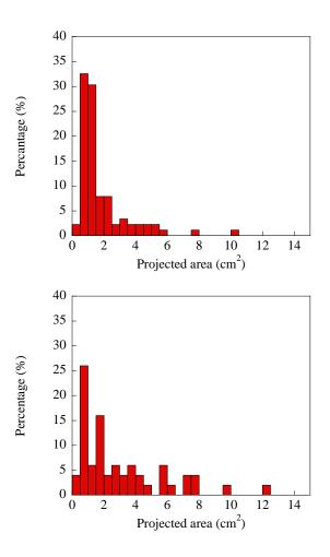
Figure 3 Size distribution of firebrands from structure; firebrand collected 18 m from structure (Top) and firebrands collected around the structure (Bottom).
