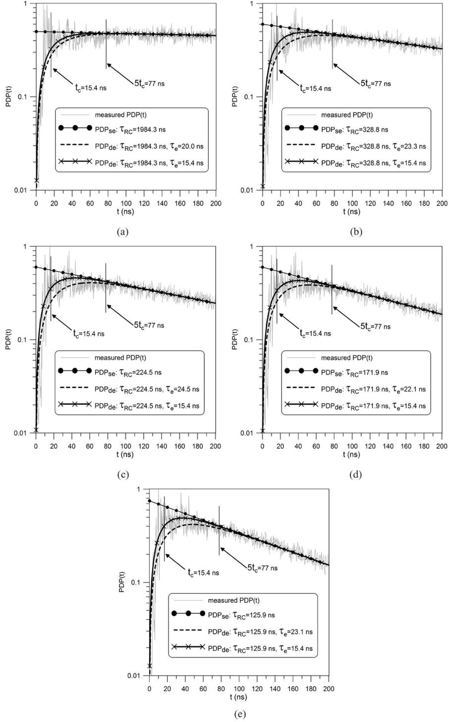
Fig. 6. Comparison of the double-exponential model to measured  $PDP(t)$ , (a) zero-absorber, (b) loading 2 (two pieces of absorber), (c) loading 3 (three pieces of absorber), (d) loading 4 (four pieces of absorber), and (e) loading 5 (five pieces of absorber).
