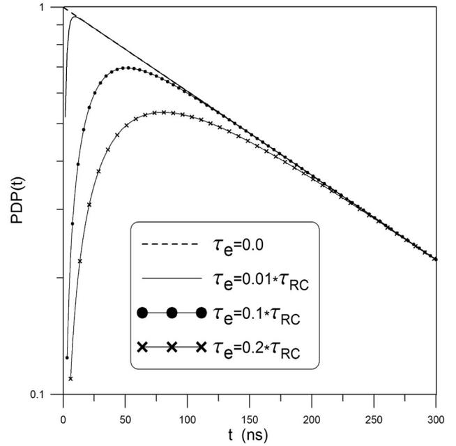
Fig. 2. Illustration of the double-exponential model for PDP( $t$ ) for various values of  $\tau_{RC}/\tau_e$ , with  $\tau_{RC} = 200$  ns.
