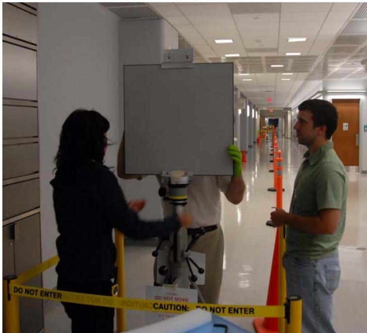
**Figure 3.** A Spectralon target being mounted on a stand.
