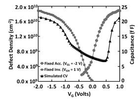
FIG. 2.  $I_{CP}$  normalized to defect density versus pulse height for the cases of fixed accumulation and fixed inversion providing a count of defects as a function of energy. Also included is a simulated CV curve.
