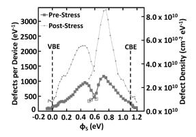
FIG. 3. Illustration of the interface state DOS obtained by differentiating the data from Fig. 2 with respect to silicon surface potential. This signature double peak response is consistent with amphoteric  $P_b$  centers.
