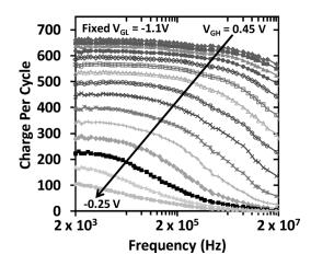
FIG. 1. The effect of insufficient interface trap filling time is illustrated by plotting charge per cycle versus CP frequency for the case of fixed accumulation. Clearly, as  $V_{GH}$  is reduced from inversion deep into depletion or the frequency is increased, an apparent loss in charge per cycle occurs. This effect must be avoided.
