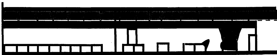
12TH FLOOR 10:33 - 1000KW - SMOKE <2 FT THICK - 200F - ZONE 2 - PLENUM DETECTOR RESPONDS
