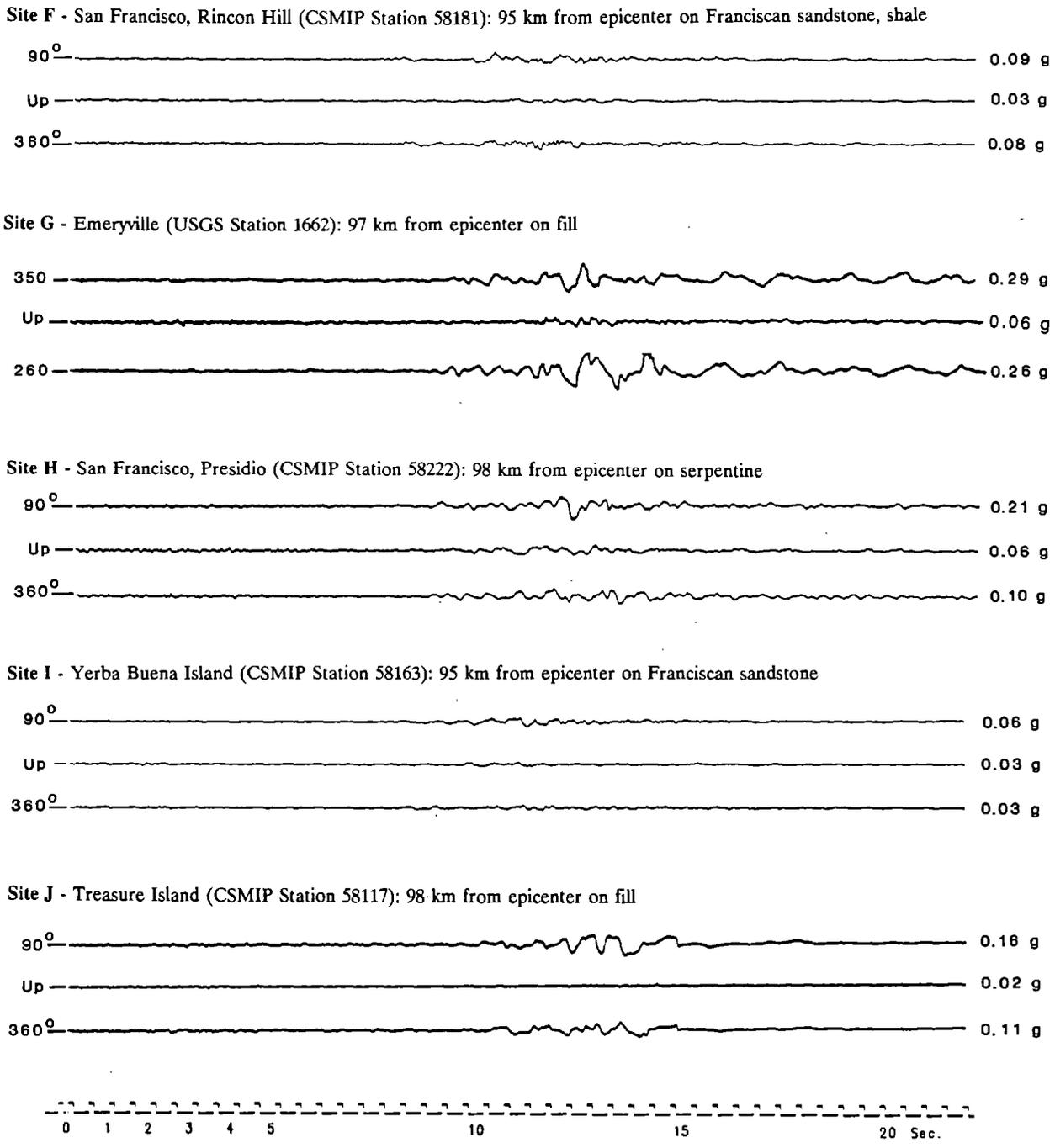
Figure 2.3.4 (Cont'd) Ground accelerations for the stations designated A-J in figure 2.3.1. The distance from the epicenter and the site geology are indicated.
