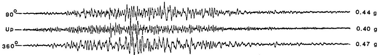
Site D - Lexington Dam, left abutment (CSMIP Station 57180): 19 km from epicenter on slate and limestone
