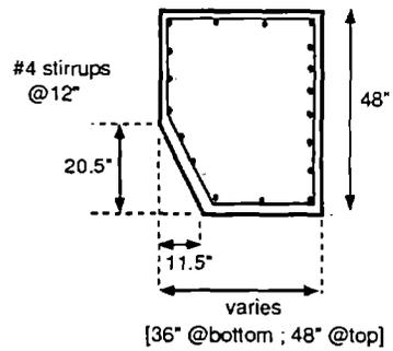
Figure 5.6.5 Structural configuration of Type 4 bents used on the elevated section of I-880.
