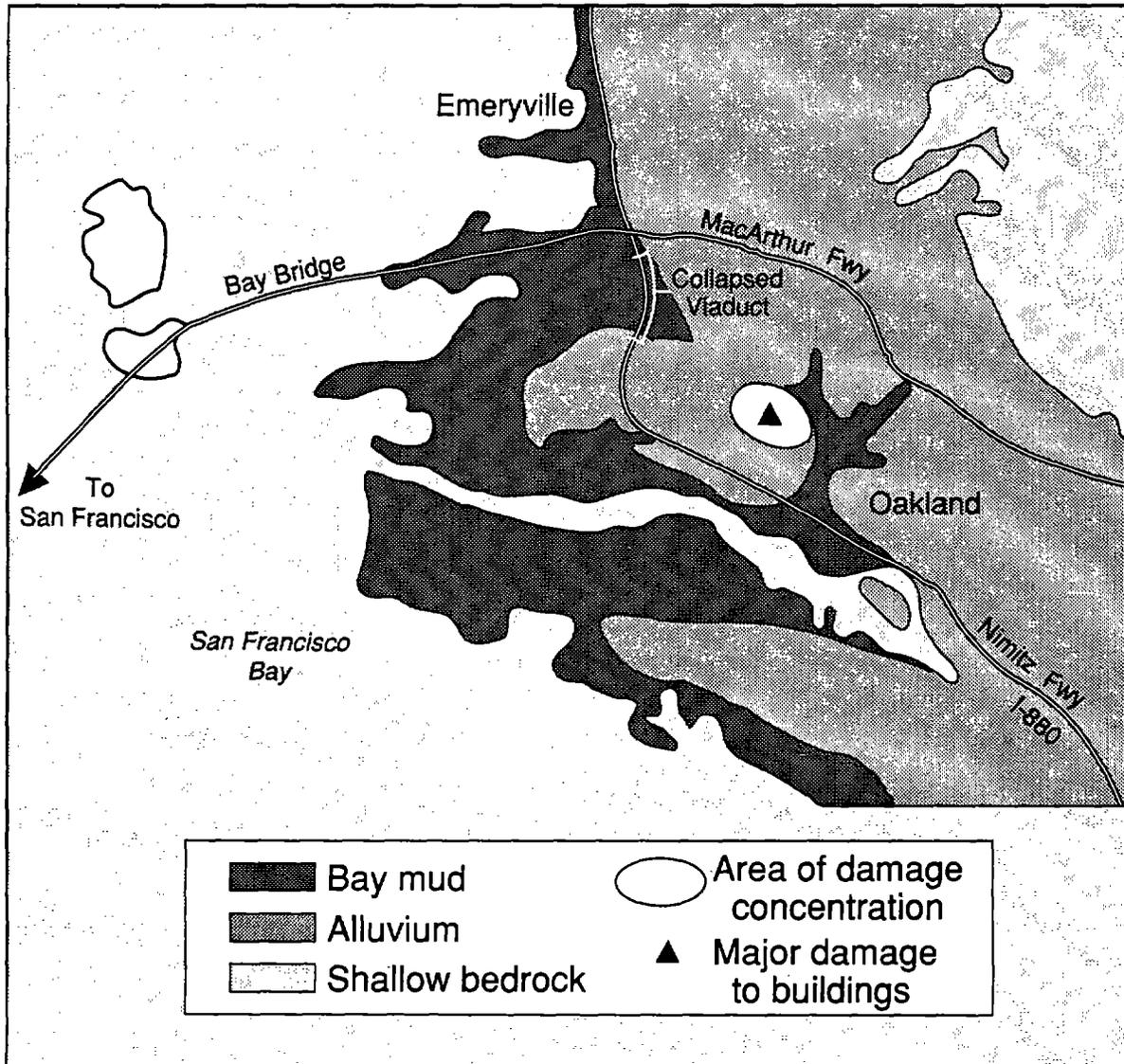
Figure 3.3.7 Surficial geology of the Oakland Area.
