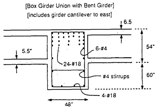
Figure 5.6.6 Structural configuration of Type 5 bents used on the elevated section of I-880.
