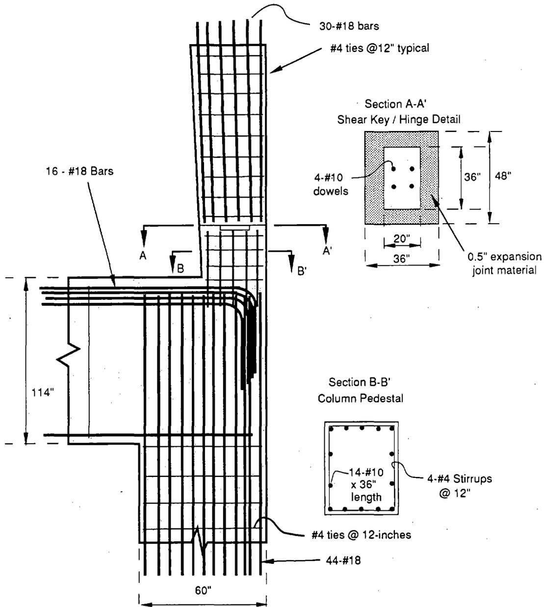
Figure 5.6.7 Reinforcement detail at the connection between the upper and lower portal frames for the Type 1 bents used in Cypress Structure, I-880.
