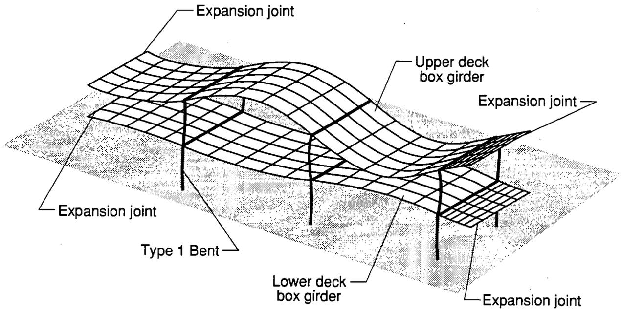
Figure 5.6.50 Vertical vibration mode shape for Cypress Structure. Period = 0.16 seconds (6.2 Hz). Boundary conditions at the ends of the spans were chosen such that the effective model included nine spans of the structure; only the central three are shown here for clarity with the termination points for the box girders occurring at the expansion joints.
