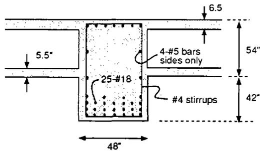
Figure 5.6.4 Structural configuration of Type 3 bents used on the elevated section of I-880.
