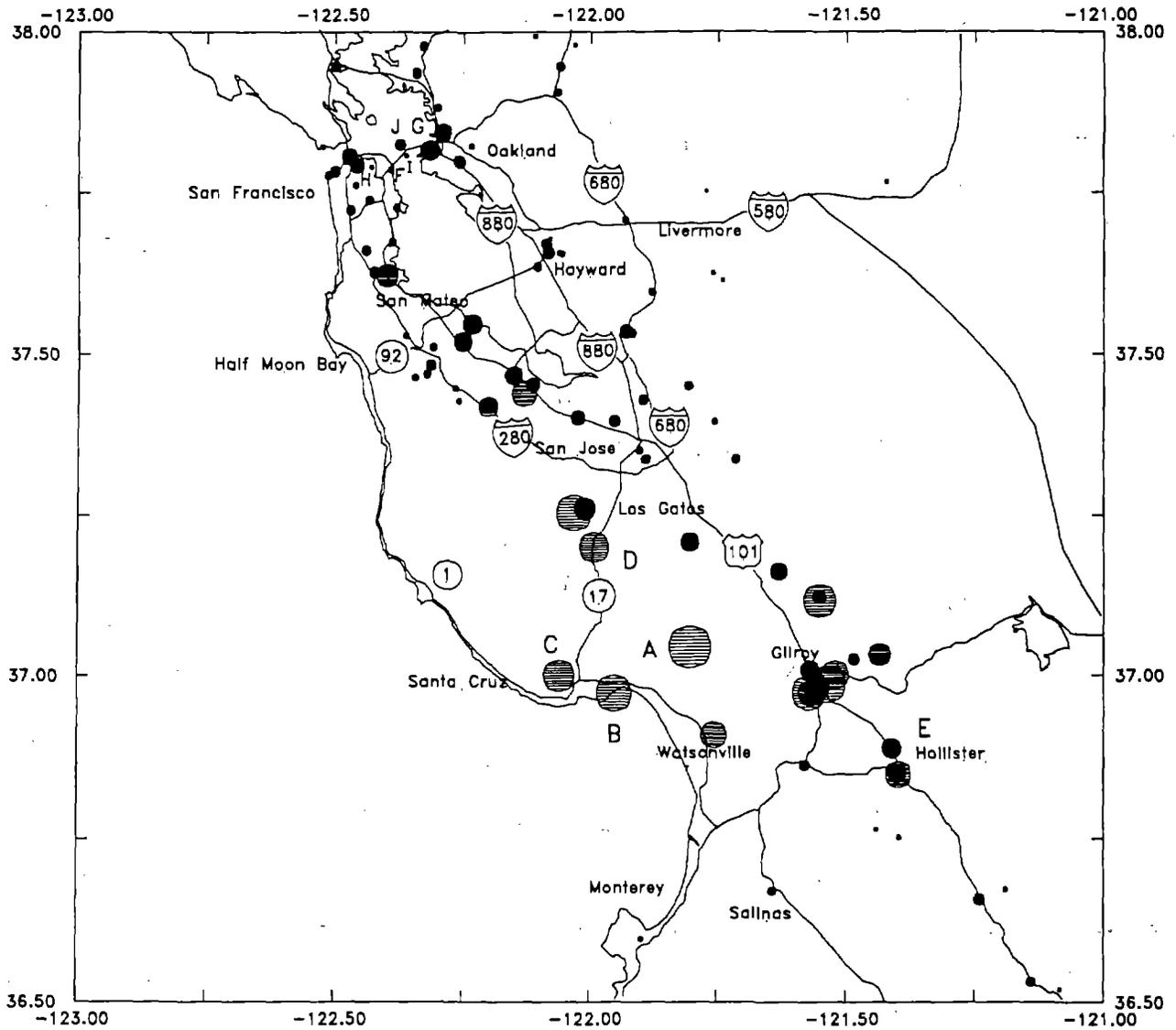
Figure 2.3.3 The relative peak horizontal acceleration is shown at each of the stations identified in figure 2.3.1 by the diameter of the circles. The largest circle at site A represents an acceleration of 0.64 g.
