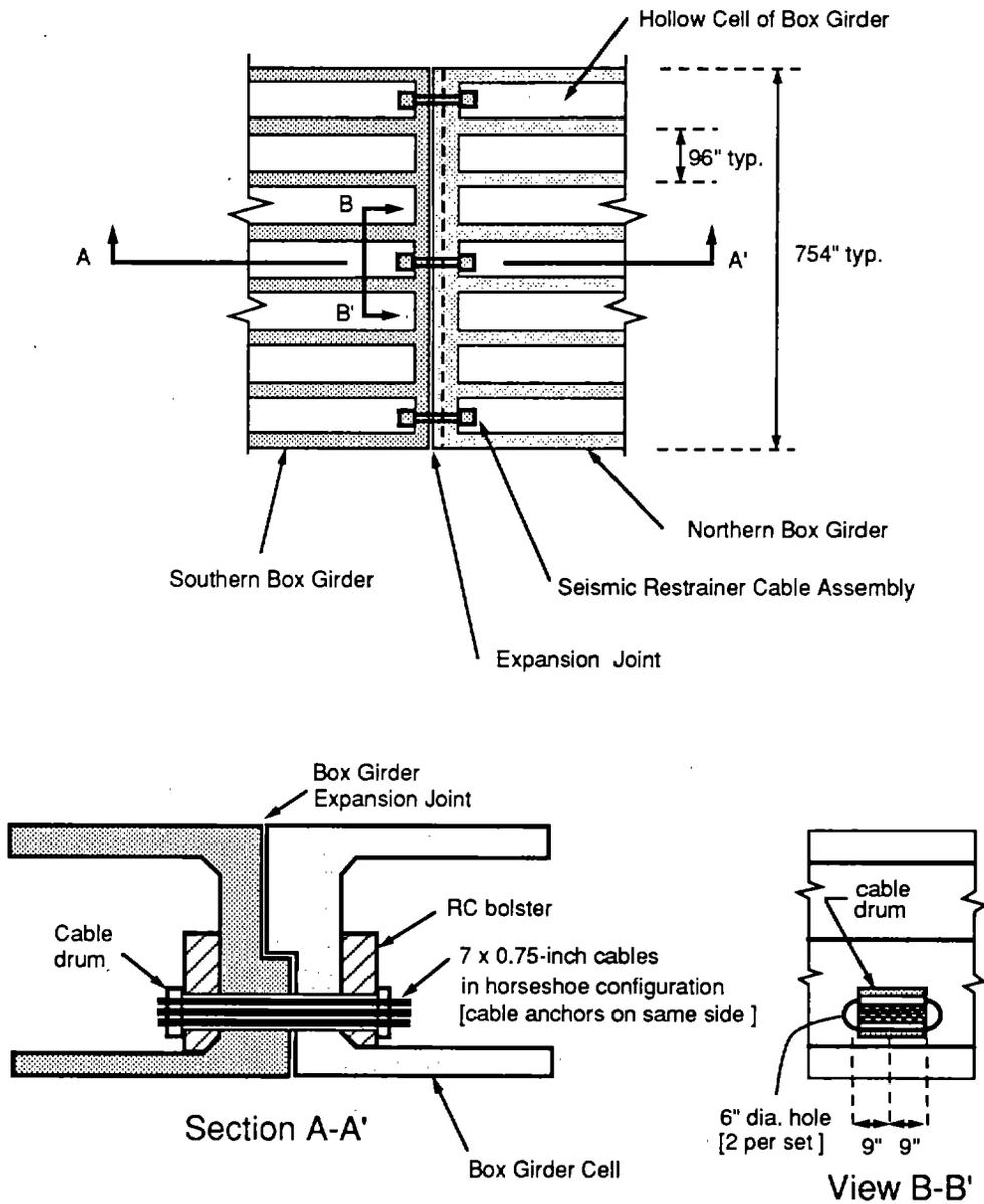
Figure 5.6.8 Detail of the Caltrans Phase I Retrofit implemented at the box girder expansion joints for Cypress Structure, I-880.
