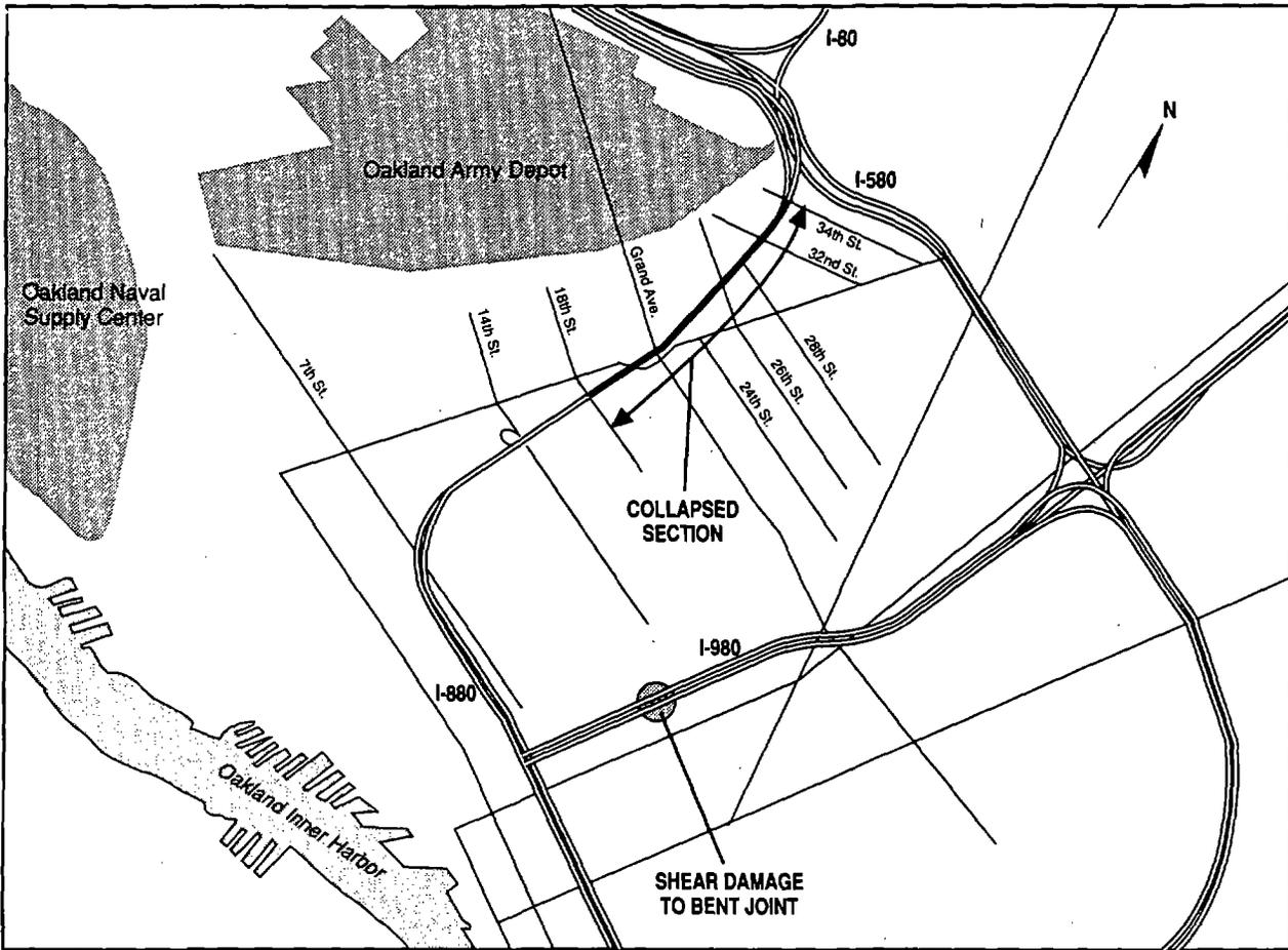
Figure 5.6.1 Map of northwest Oakland depicting the location of the collapse of I-880 and bent damage to I-980.
