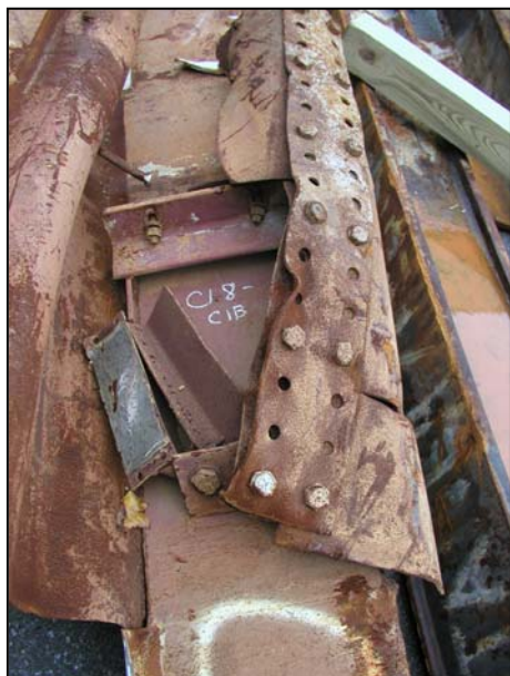
Figure B-5. Floor truss connectors found on recovered panel C-18 (B230: 93-96) from WTC 2. Shown are connectors found on column 231 at different floor levels.
