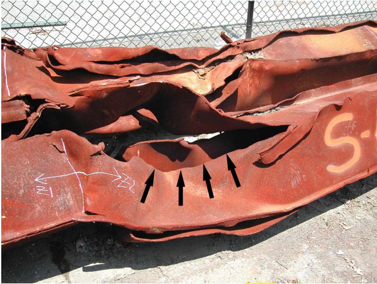
Figure 9. Ruptures of fillet welds through parent material HAZ on possible fire-effected region of Piece S-10
