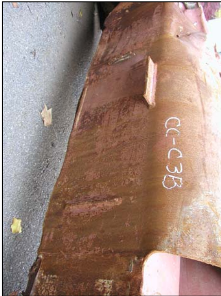
Figure B-17. Floor truss connectors found on recovered panel CC (A124: 70-73) from WTC 1. Shown are connectors found on column 123 at different floor levels (cont.).
