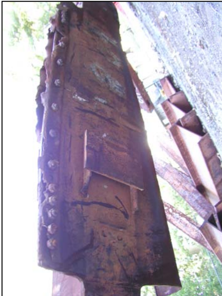
Figure B-1. Floor truss connectors found on recovered panel ASCE-2 (B330: 40-43) from WTC 2. Shown are connectors found on column 329 at different floor levels (cont.).
