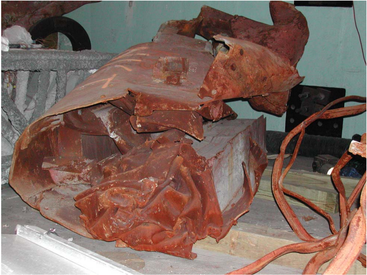
Figure 22. Piece K-1, which has collapsed in compression
