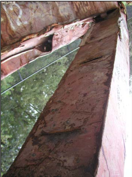
Figure B-33. Floor truss connectors found on recovered panel N-12 (A206: 92-95) from WTC 1. Shown are connectors found on column 206 at different floor levels (cont.).
