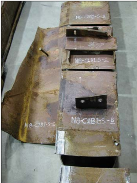
Figure B-30. Floor truss connectors found on recovered panel N-8 (A142: 97-100) from WTC 1. Shown are connectors found on column 143 at different floor levels.
