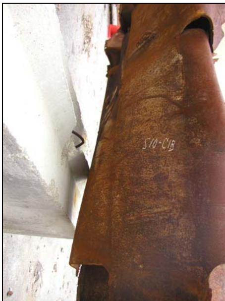
Figure B-39. Floor truss connectors found on recovered panel S-10 (A224: 92-95) from WTC 1. Shown are connectors found on column 225 at different floor levels.
