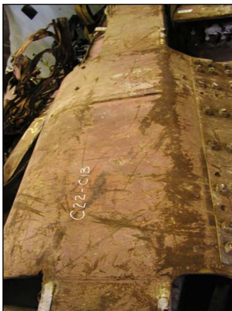
Figure B-6. Floor truss connectors found on recovered panel C-22 (A157: 93-96) from WTC 1. Shown are connectors found on column 158 at different floor levels.
