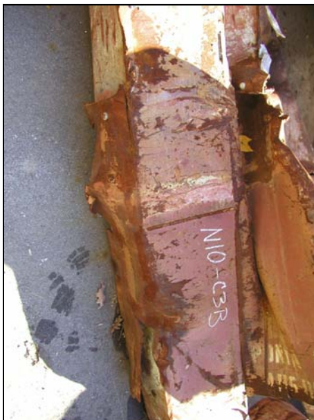
Figure B-32. Floor truss connectors found on recovered panel N-10 (A115: 89-92) from WTC 1. Shown are connectors found on column 114 at different floor levels (cont.).
