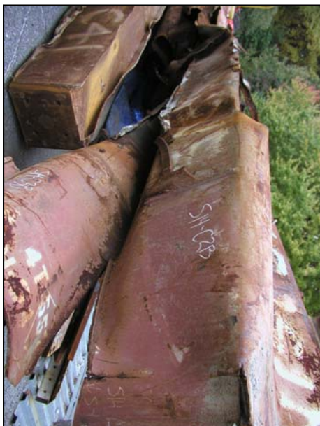
Figure B-40. Floor truss connectors found on recovered panel S-14 (B218: 91-94) from WTC 2. Shown are connectors found on column 218 at different floor levels (cont.).
