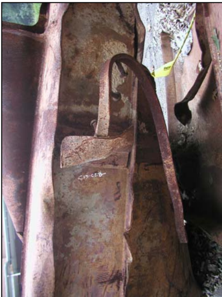
Figure B-3. Floor truss connectors found on recovered panel C-13 (B200: 90-92) from WTC 2. Shown are connectors found on column 200 at different floor levels (cont.).
