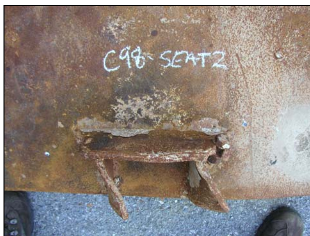
Figure C-5. Sample C-98, channel with two seats.
