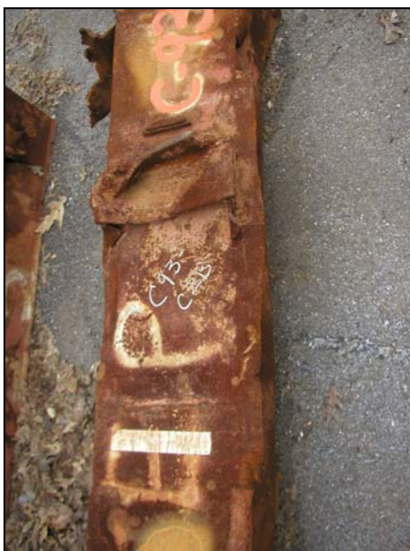
Figure B–15. Floor truss connectors found on recovered panel C-93 (A339: 99-102) from WTC 1. Shown are connectors found on column 339 at different floor levels (cont.).
