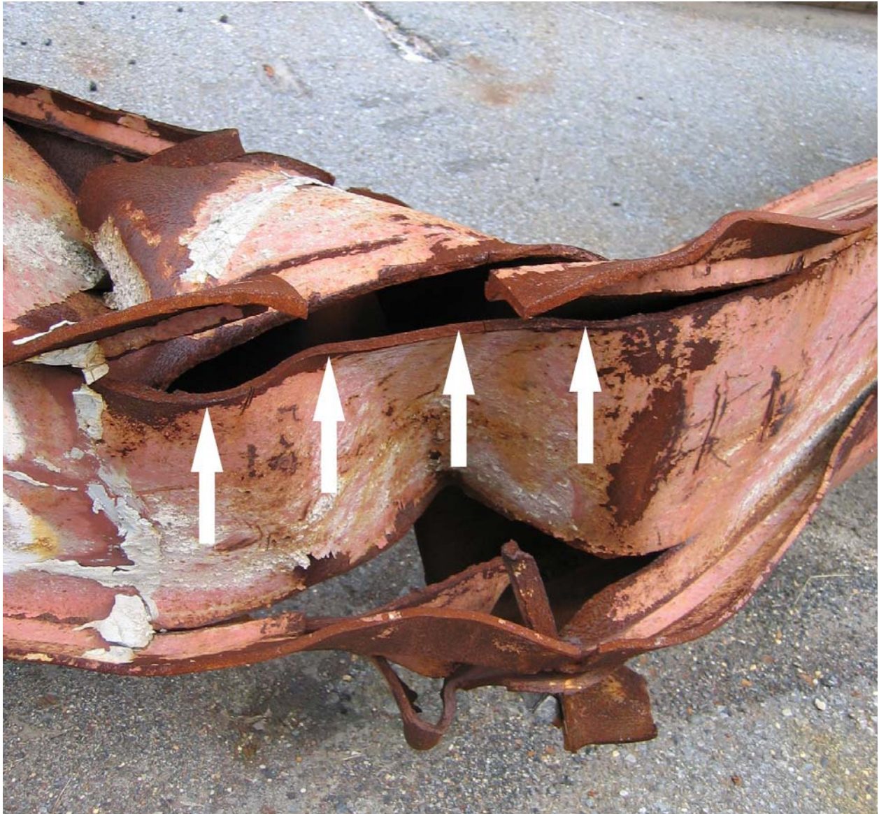
Figure 10. Ruptures of fillet welds through parent material HAZ (at arrows) on probable mechanically pinched zone on Piece C-40 (ruptures through parent material away from welds are also observable in the photo)
