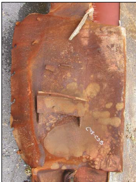
Figure B-11. Floor truss connectors found on recovered panel C-48 (B442: 91-94) from WTC 2. Shown are connectors found on column 441 at different floor levels (cont.).
