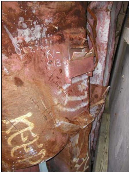
Figure B-18. Floor truss connectors found on recovered panel K-1 (A209: 97-100) from WTC 1. Shown are connectors found on column 210 at different floor levels.
