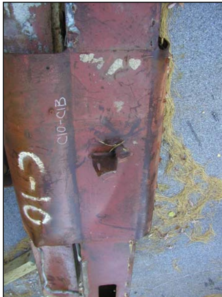
Figure B-2. Floor truss connectors found on recovered panel C-10 (A451: 85-88) from WTC 1. Shown are connectors found on column 452 at different floor levels.
