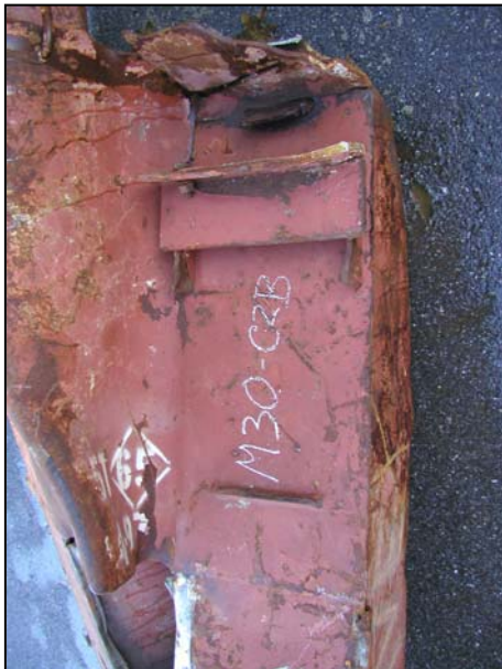
Figure B-27. Floor truss connectors found on recovered panel M-30 (A133: 94-97) from WTC 1. Shown are connectors found on column 133 at different floor levels (cont.).
