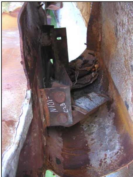
Figure B-36. Floor truss connectors found on recovered panel N-101 (A133: 100-103) from WTC 1. Shown are connectors found on column 133 at different floor levels (cont.).
