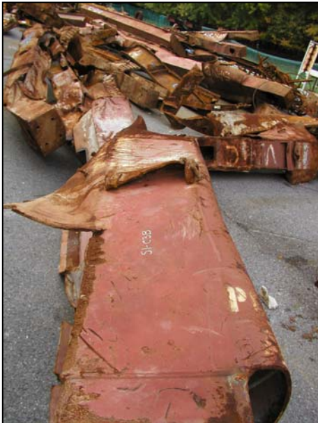
Figure B–37. Floor truss connectors found on recovered panel S-1 (A433: 79-82) from WTC 1. Shown are connectors found on column 432 at different floor levels (cont.).
