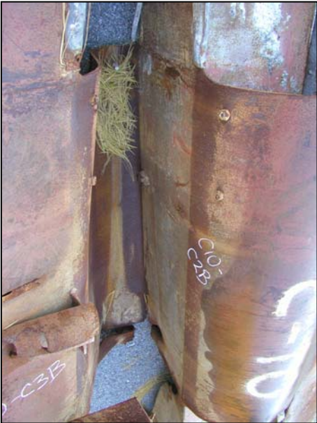
Figure B-2. Floor truss connectors found on recovered panel C-10 (A451: 85-88) from WTC 1. Shown are connectors found on column 451 at different floor levels (cont.).
