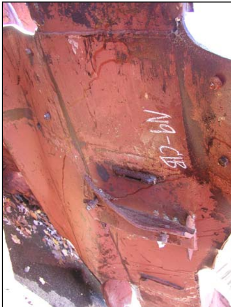
Figure B-31. Floor truss connectors found on recovered panel N-9 (A154: 101-104) from WTC 1. Shown are connectors found on column 155 at different floor levels.
