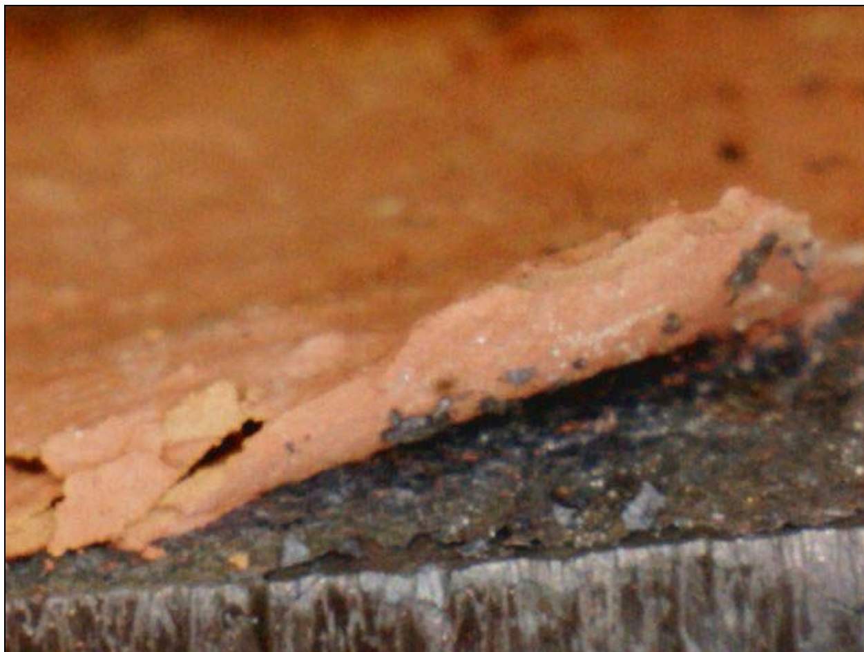
Figure D–4. Formation of a black scale between paint and steel after exposure greater than 650 °C. Paint readily spalled.
