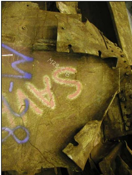
Figure B–26. Floor truss connectors found on recovered panel M-28 (B345: 98-101) from WTC 2. Shown are connectors found on column 346 at different floor levels.
