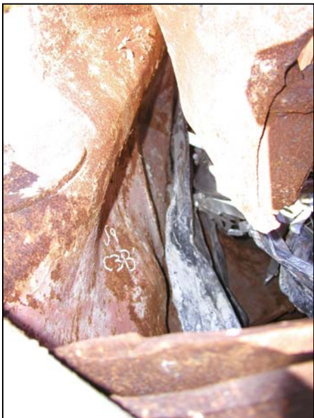
Figure B-38. Floor truss connectors found on recovered panel S-9 (A133: 97-100) from WTC 1. Shown are connectors found on column 132 at different floor levels (cont.).
