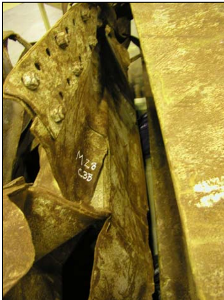
Figure B-26. Floor truss connectors found on recovered panel M-28 (B345: 98-101) from WTC 2. Shown are connectors found on column 344 at different floor levels (cont.).
