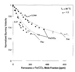
Figure 1. Normalized burning velocity of premixed  $CH_4/O_2/N_2$  flames inhibited by ferrocene (open symbols) and Fe(CO)<sub>5</sub> (closed symbols) for  $X_{O_2,O_x}$  =0.21 and 0.244, together with modeling predictions (dotted lines).
