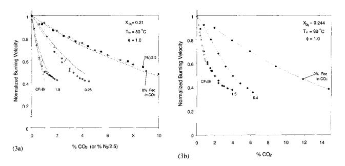
Figure 3. Normalized burning velocity of  $CH_4/O_2/N_2$  flames, a)  $X_{O_2,O_x} = 0.21$ , b)  $X_{O_2,O_x} = 0.244$ , inhibited by  $CO_2$ , by  $CO_2$ -ferrocene blends, and by  $CF_3Br$ . The equivalent percentage of ferrocene in  $CO_2$  (which is constant for each curve) is given. The solid lines are curve fits through the data, and the dotted lines, the calculated results. Data for nitrogen are included in (a) by dividing %  $N_2$  by 2.5.
