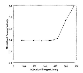
Figure 2. The normalized burning velocity of stoichiometric  $CH_4/O_2/N_2$ flames at 400 ppm of Fec as a function of the activation energy of the one-step ferrocene decomposition reaction.
