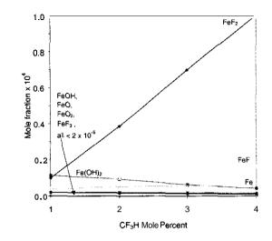
Figure 6. Equilibrium mole fraction of active inhibiting species (Fe, FeO, FeOH, Fe(OH)<sub>2</sub>) and iron-fluorine species with 1% to 4% CF<sub>3</sub>H (containing 0.35% ferrocene) added to a stoichiometric methane-air reaction mixture.
