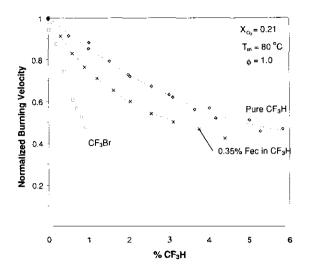
Figure 5. Normalized burning velocity of premixed  $CH_4/O_2/N_2$  flames inhibited by pure  $CF_3H$  and by  $CF_3H$  with 0.35% ferrocene, together with data for  $CF_3Br$ . Lines are curve fits to the data.
