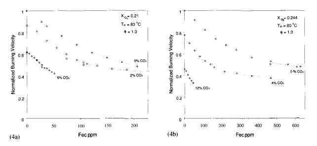
Figure 4. Normalized burning velocity of  $CH_4 / N_2 / O_2$  flames, a.)  $X_{O_2,O_3} = 0.21$ , b.)  $X_{O_2,O_3} = 0.244$ , with 0, 2, and 6, or 0, 6, and 12 mole percent of CO<sub>2</sub>, respectively, added to the reactant stream, as a function of added ferrocene (lines are curve fits to the experimental data).
