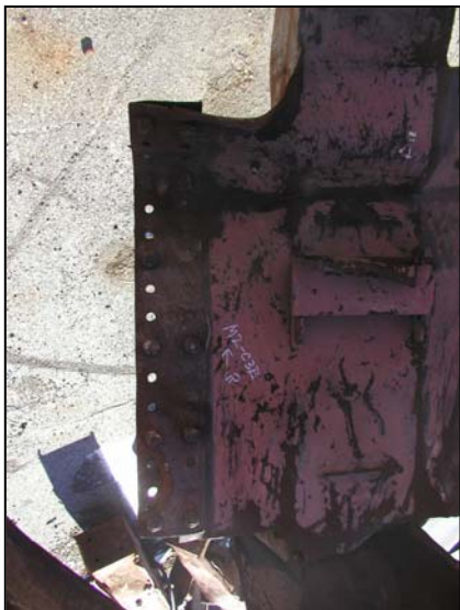
Figure 6–25. Photographs of recovered spandrel connections from sample M-2 (A130: 96-99) (continued).
