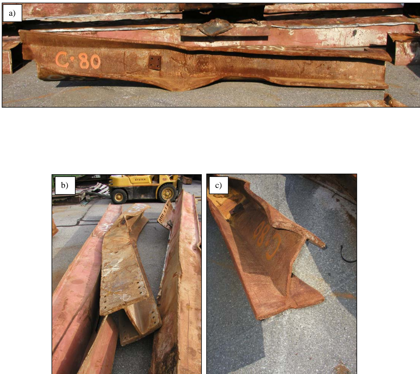
Figure 6–30. Core column C-80 (603A: 92-95). a) Overall view of recovered column, b) view of connection in the 92nd floor region, failure as a result of bolt fracture, and c) torn end of column near the 94th floor region.
