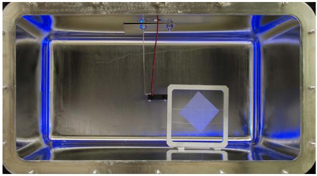
Figure 1. Reference film in NIST 50 L stainless steel chamber.
