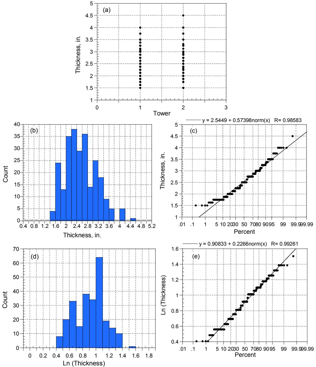
**Figure 4-4. (a) Dotplot of individual thickness measurements on floor trusses from Port Authority Construction Audit Reports, (b) histogram of thickness measurements, (c) normal probability plot of thickness measurements, (d) histogram of natural logarithms of thickness measurements, and (e) normal probability plot of natural logarithm of thickness measurements.**
