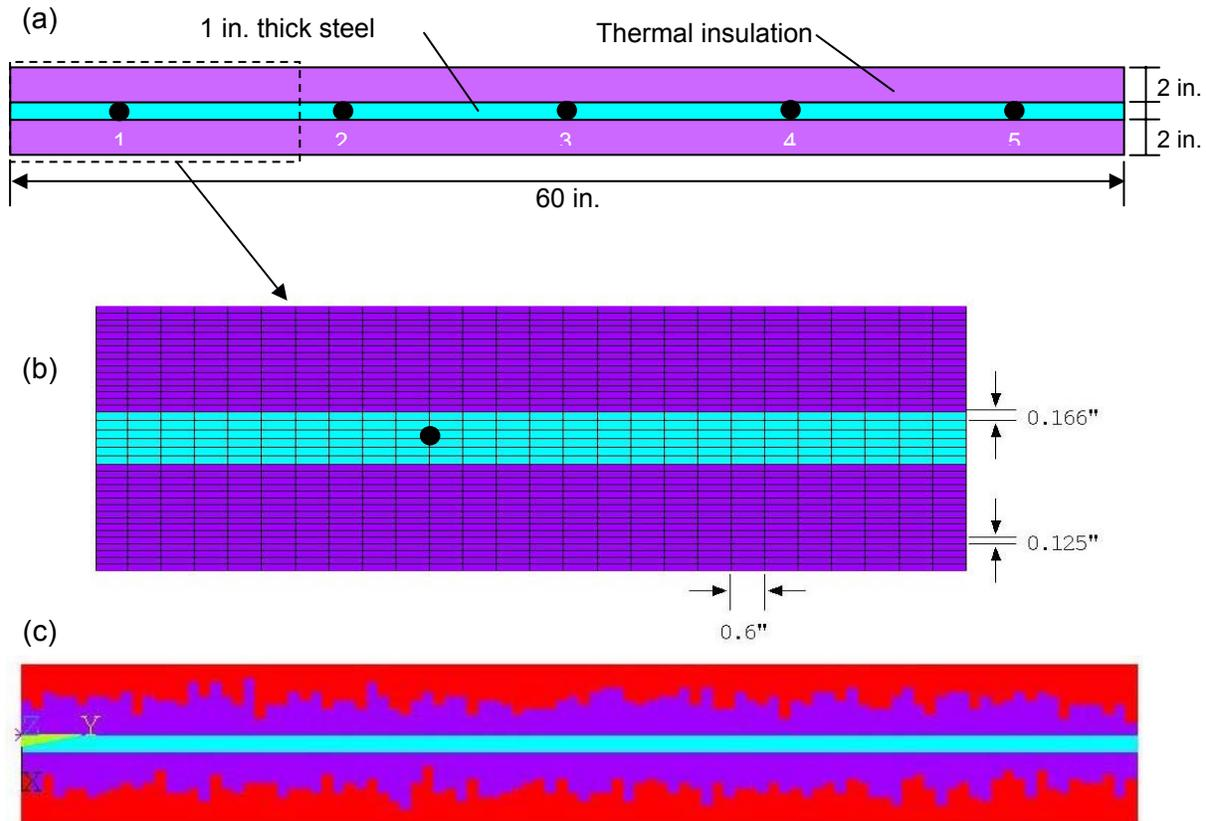
**Figure 5–1. Model used to study effects of SFRM thickness and variability of thickness on steel temperature: (a) physical model used in analyses (points 1 to 5 are locations where temperatures are monitored), (b) finite element mesh used to represent physical model, and (c) finite element model to represent variable thickness of SFRM (purple) (the elements in red represent material of high thermal conductivity).**
