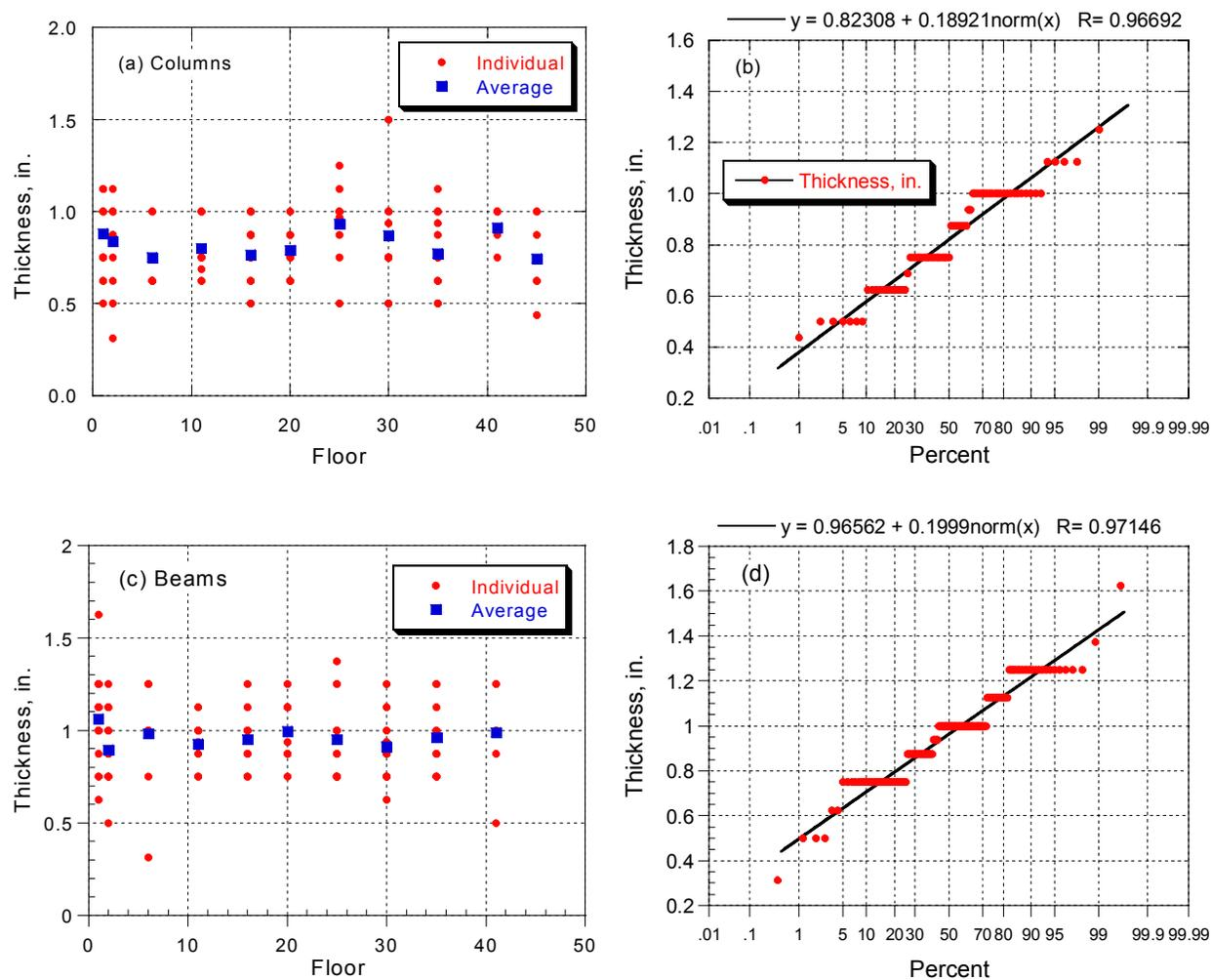
**Figure 4-6. Thickness of re-applied SFRM in elevator shaft 10/11 of WTC 1: (a) Individual and average thickness for core columns, (b) normal probability plot of individual measurements on columns, (c) individual and average thickness for core beams, and (d) normal probability plot of individual measurements on beams.**
