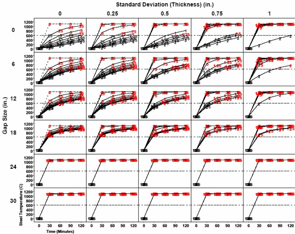
**Figure 5–6. Example of plot matrix from sensitivity study of the effects of missing SFRM and variability of SFRM thickness on steel temperature. Each graph is a temperature history of the steel at point #2 (see Fig. 5-5 for location) for different thicknesses of SFRM.**
