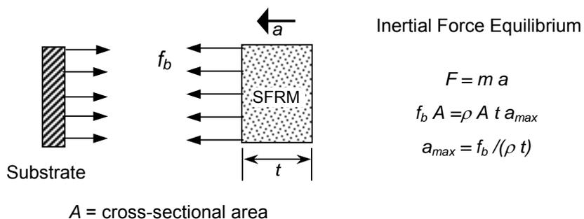
**Figure 7–28. Derivation of acceleration to dislodge SFRM from planar substrate.**
