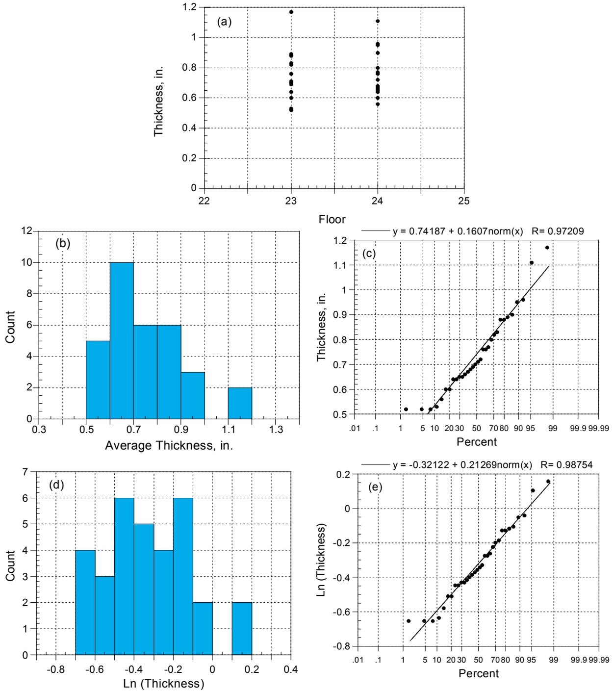
**Figure 4-1. (a) Dotplot of average thickness from floor trusses for floors 23 and 24, (b) histogram of average thickness, (c) normal probability plot of average thickness, (d) histogram of natural logarithm of average thickness, and (e) probability plot of natural logarithm of average thickness.**
