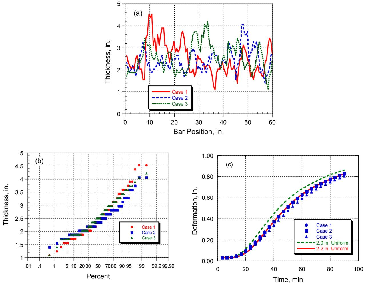
**Figure 5–8. (a) Randomly generated thickness profiles with average thickness of 2.5 in. and standard deviation of 0.6 in., (b) normal probability plots of thickness values, and (c) deformation of 1 in. bar compared with deformation for uniform thickness of thermal insulation.**
