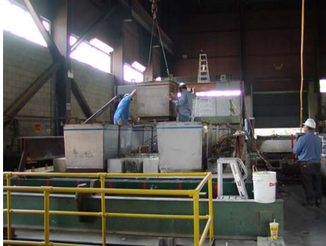
Figure 3–5. 35 ft span test assembly loaded with concrete blocks and water-filled containers.
