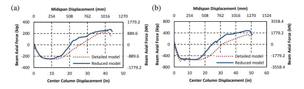
Fig. 6. Beam axial forces versus vertical displacement of center stub column for (a) IMF specimen and (b) SMF specimen
