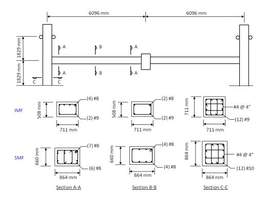
Fig. 2. Dimensions and reinforcement details of test specimens
