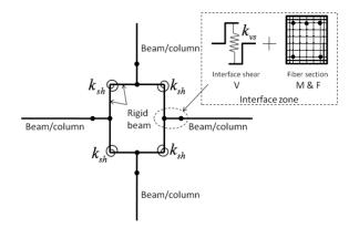
Fig. 1. Reduced beam-to-column connection model
