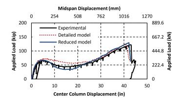
Fig. 4. Vertical load versus vertical displacement of center stub column for the IMF specimen
