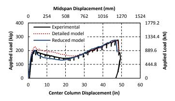
Fig. 5. Vertical load versus vertical displacement of center stub column for the SMF specimen
