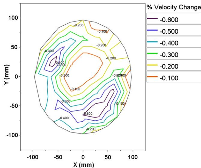
Fig. 3. Composite contour map of the within wafer variation of the change in sound velocity of blanket  $\text{SiO}_x$  on a 200 mm wafer.
