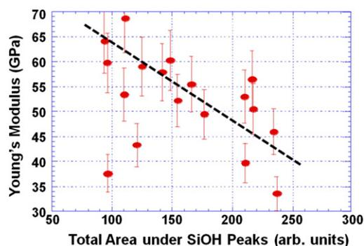
Fig. 4. Correlation of Young's modulus with relative local SiOH concentration from various dies from a typical  $\text{SiO}_2$  wafer.
