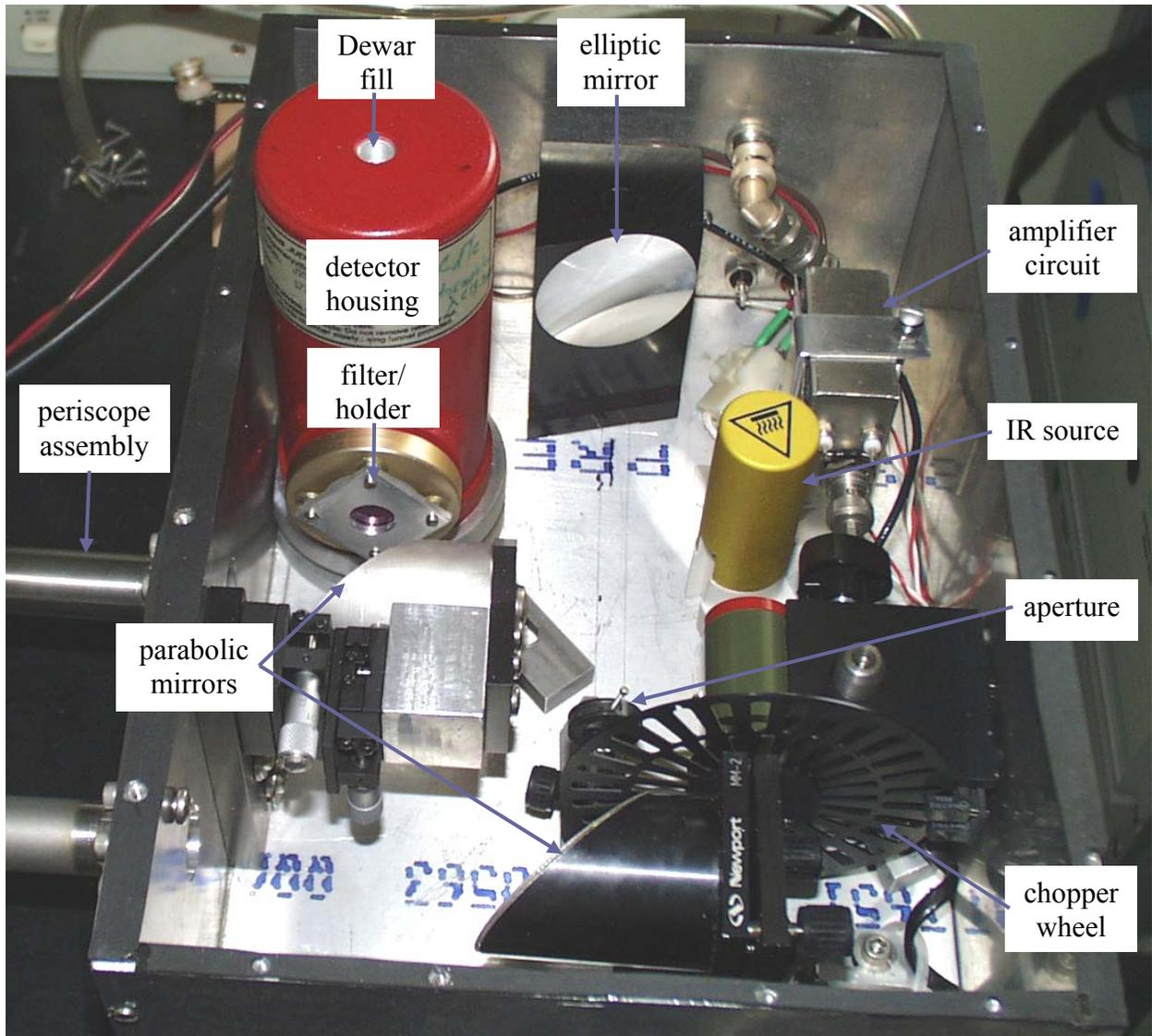
Figure 2. A photographic view from the opposite direction as Fig. 1 of the DIRRACS II interior showing the general layout including relative sizes and positions of components.
