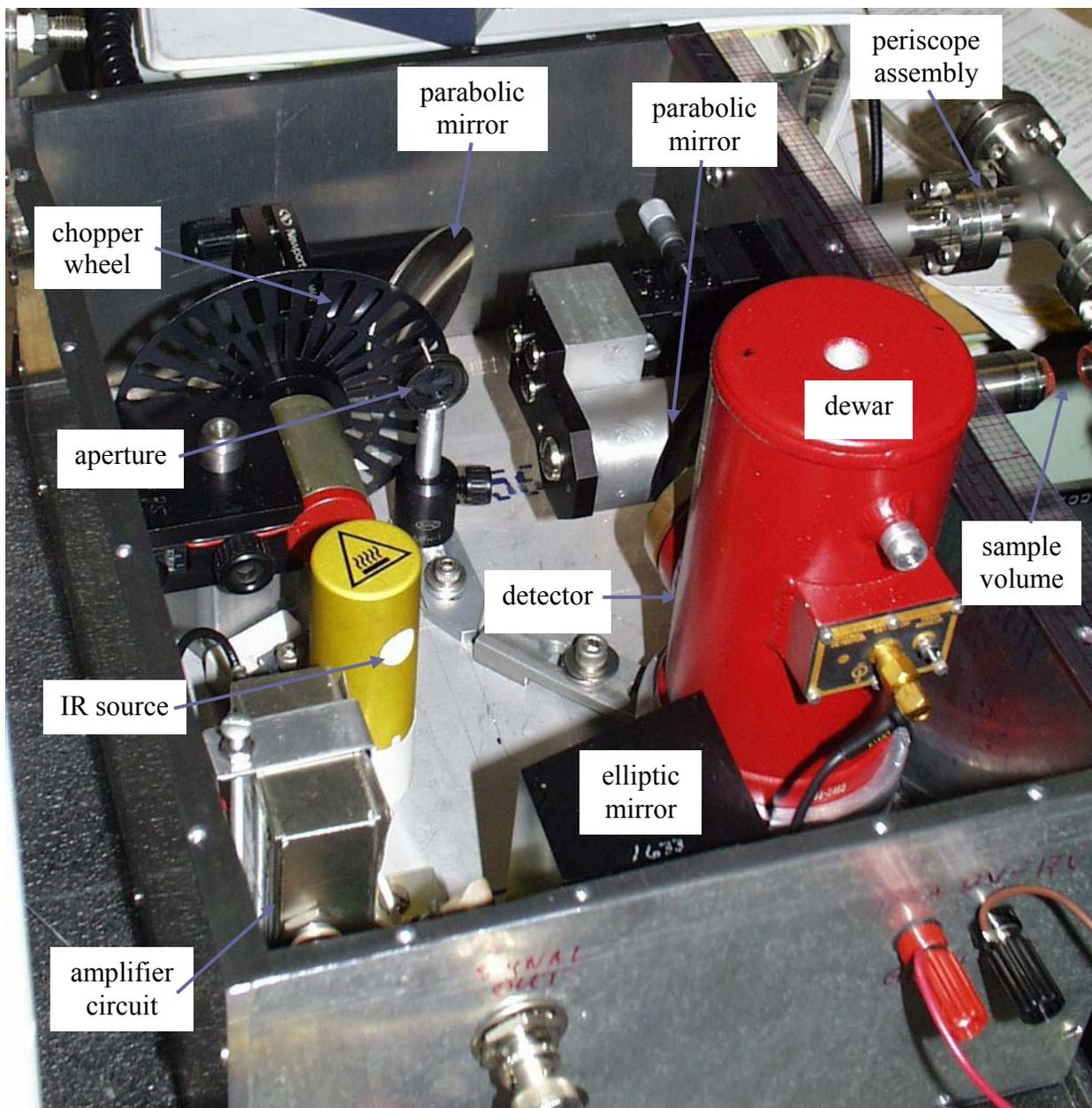
Figure 1. A photographic view of the DIRRACS II interior showing the general layout including relative sizes and positions of components.
