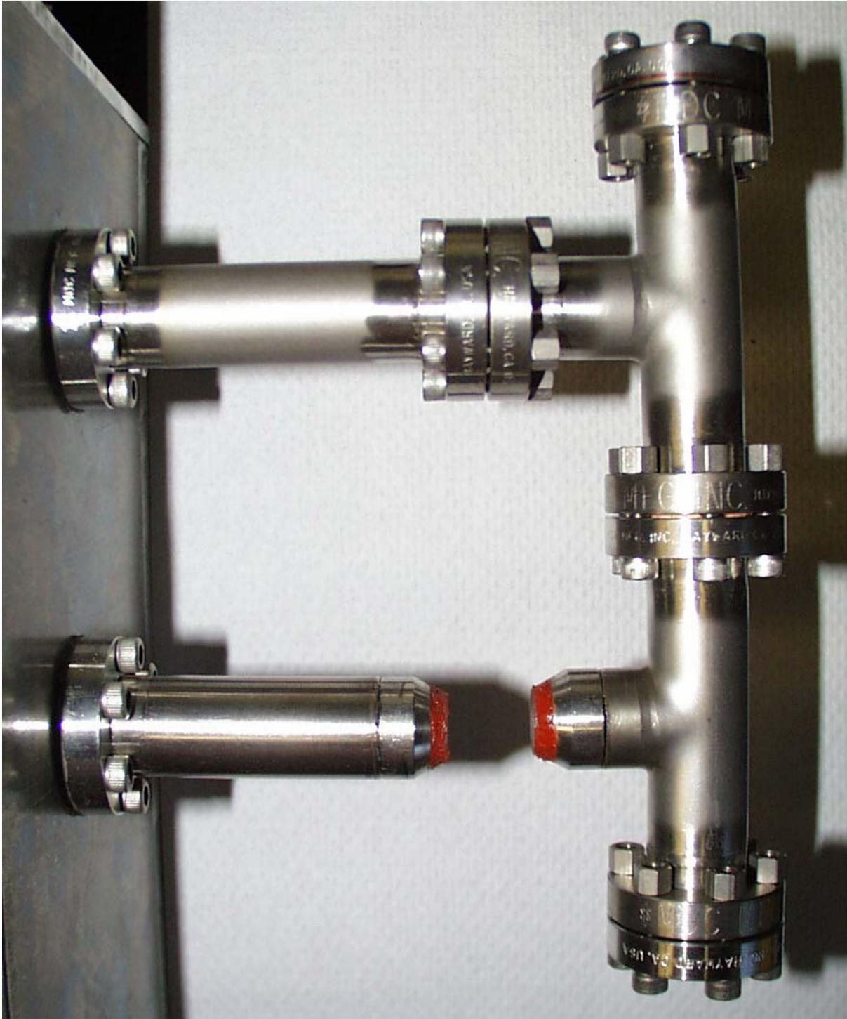
Figure 9. A photograph of the periscope attached to the DIRRACS II chassis.
