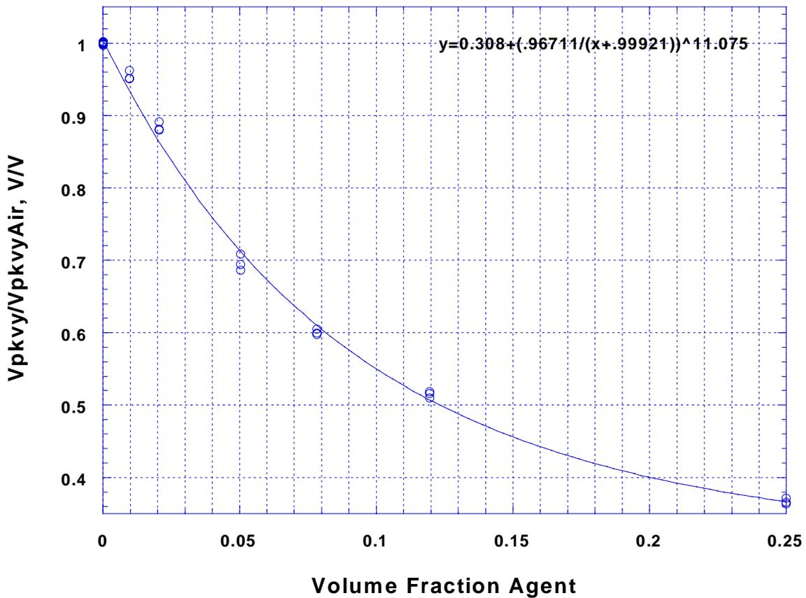
Figure 20. A typical calibration plot of average normalized peak-to-valley signals versus the volume fraction of HFC-125. Error bars for the averages are smaller than the symbols.
