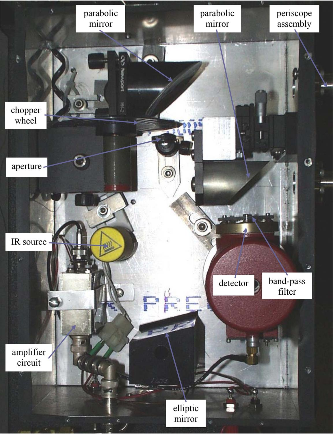
Figure 3. A photograph of the DIRRACS II interior from above showing the optical components.
