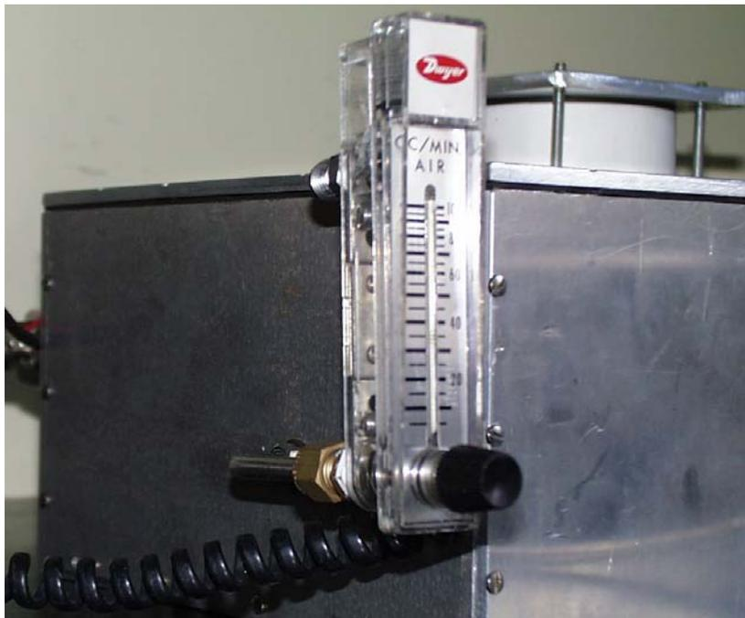
Figure 7. A photograph of the side of the chassis where the N<sub>2</sub> purge exhausts and its flow is monitored and where the chopper controller cable enters the chassis.
