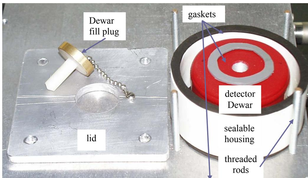
Figure 8. A photograph of the detector Dewar sealable housing, tightening rods, lid, gaskets, and Dewar fill plug.
