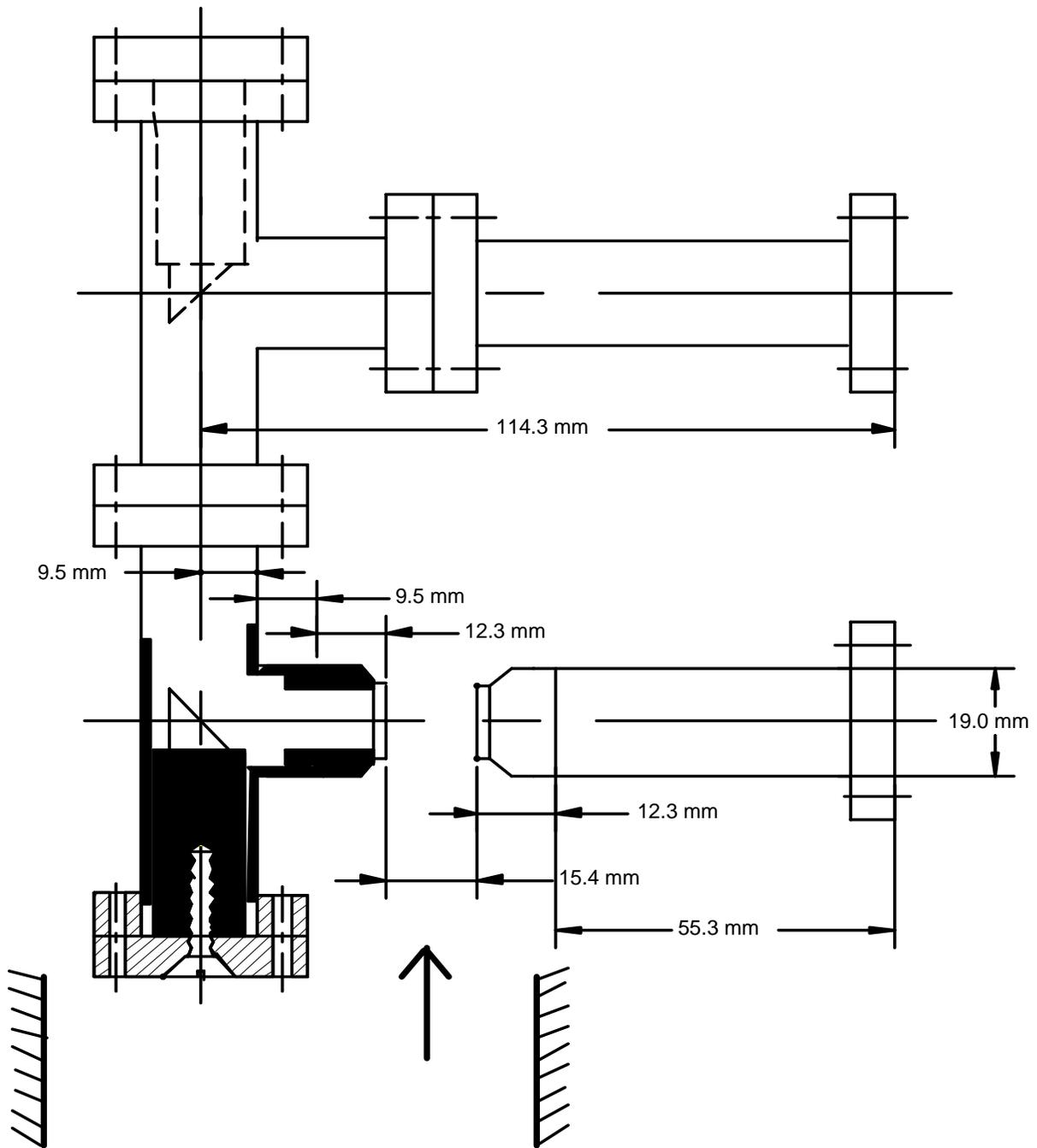
Figure 10. A drawing of the periscope assembly.
