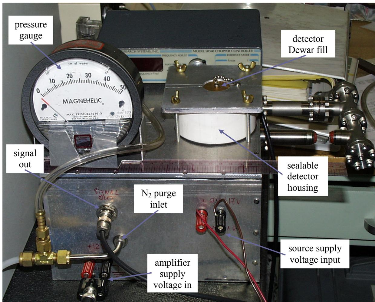
Figure 5. A photograph of the DIRRACS II chassis showing the electrical and gas connections.
