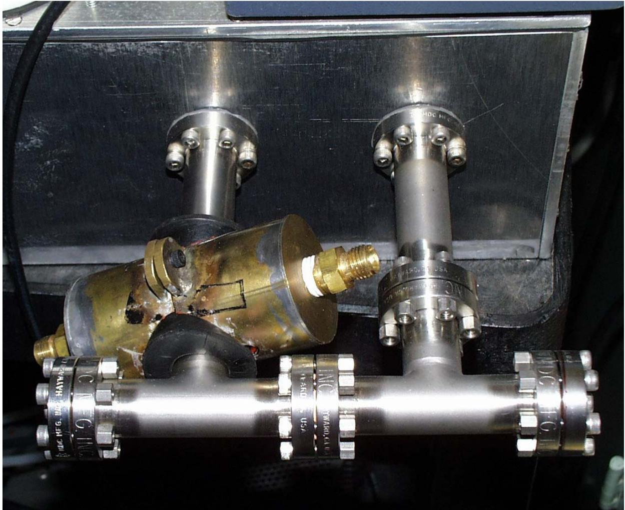
Figure 19. A photograph of the calibration cell covering the sample volume of the periscope assembly to provide known mixtures of agent and air to the instrument.
