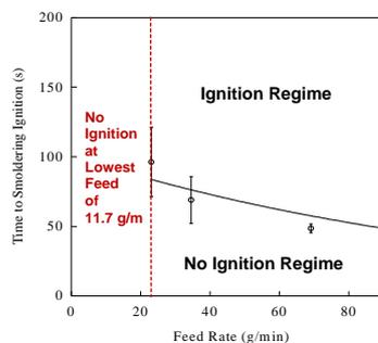
**Figure 2.** Ignition regime map (smoldering ignition - SI) as a function of glowing feed rate for wind tunnel speed of 6 m/s.
