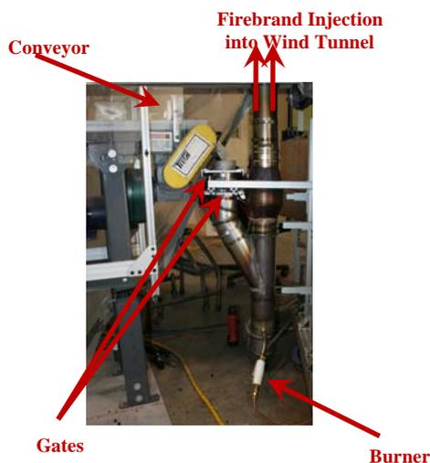
**Figure 1** Schematic of NIST Continuous Feed Baby Dragon (side view) interfaced with bench scale wind tunnel.
