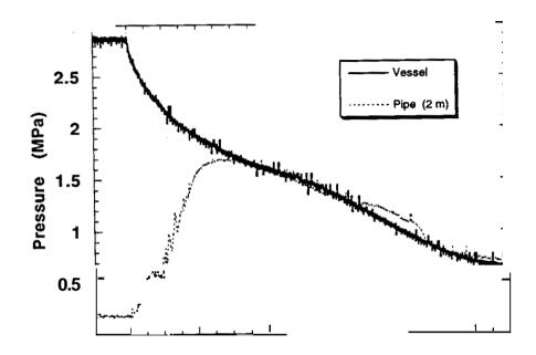
Figure 2. Pressure traces for HFC-227ea tested at a 50% fill condition, pressurized to 2.8 MPa with no make-up nitrogen addition.
