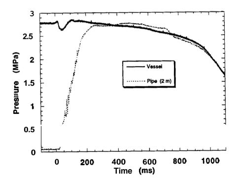
Figure 3. Pressure traces for HFC-227ea tested at a 50% 611 condition, pressurized to 2.8 MPa with make-up nitrogen addition.
