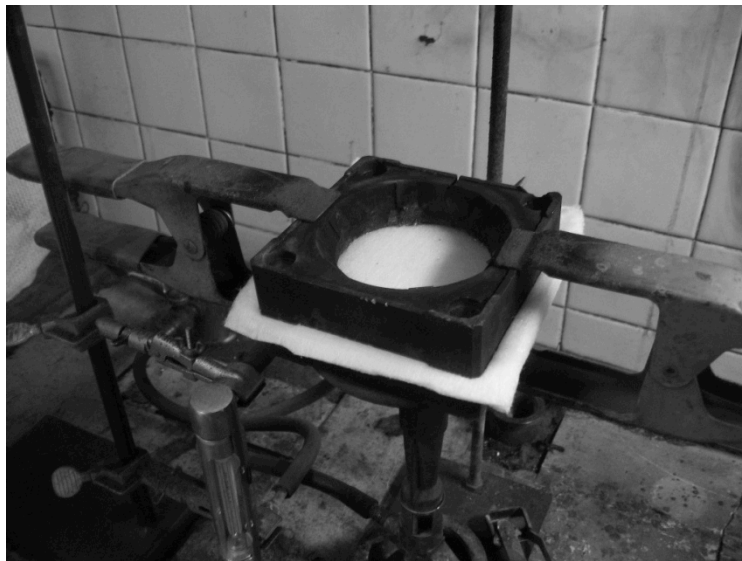
Figure 6. Meeker burner testing set up for studying char characteristics.
