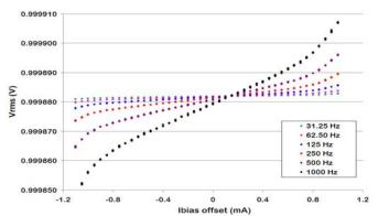
Fig. 2. PJVS rms voltage after full correction algorithm has been applied, including the final analysis that incorporates measurement bandwidth, rise time, and harmonic spectrum.
