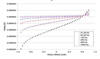
Fig. 1. PJVS rms voltage measured by a digitizer and corrected for noise, gain, and nonlinearity, but not measurement bandwidth (i.e., some of the waveform harmonics are outside the digitizer cutoff frequency).
