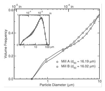
Fig. 1: PSD plotted as a volume frequency or probability distribution of Type I OPC produced from two different mills, each producing the same nominal Blaine fineness. The greater fraction of particles in the size range of 2 to 10 µm makes the cement from Mill A have a water demand that is 10 L/m<sup>3</sup> (2 gal./yd<sup>3</sup>) higher than the cement from Mill B. The inset shows the full PSD. Variation in the PSD over six repeated measurements is less than the size of the symbol in the plots
