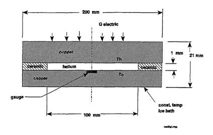
Figure 1. Schematic of conduction apparatus (elevation).
