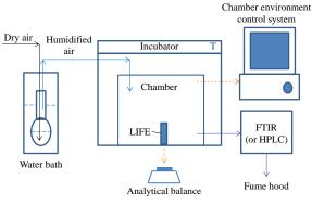
Figure 2: System for chamber test
