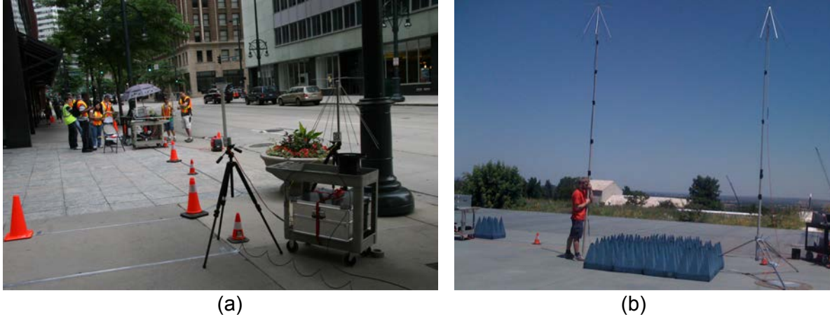
Figure 5.4: Reference measurements made in two environments. (a) Denver urban canyon, with high-frequency-band antennas placed approximately 4 m apart and 1.5 m high. (b) NIST open-area test site, with low-frequency-band antennas placed 3 m apart and 5 m high.
