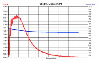
and an energy of 18 J  $\pm$  0.1 J. For low- and high-energy specimens, the uncertainty in maximum force is equivalent or better than the uncertainty in absorbed energy.
