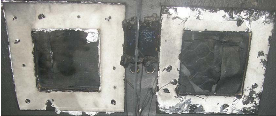
Figure 39: Thermal/mechanical damage to exterior of FFPE sample with PCM (left) and unmodified FFPE (right) after experiment two.
