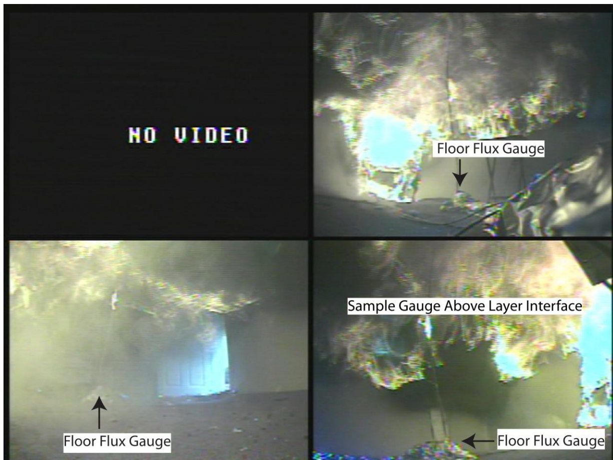
Figure 20: Video frame capture of compartment conditions immediately prior to suppression, with locations of total HF gauges indicated
