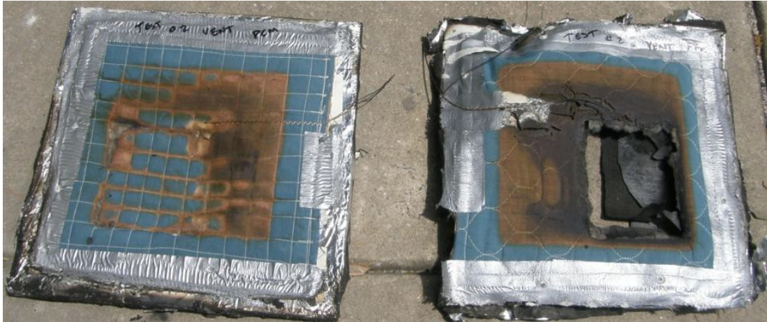
Figure 37: View of the interior liner for the FFPE with PCM (left) and the unmodified FFPE (right) after Experiment 2
