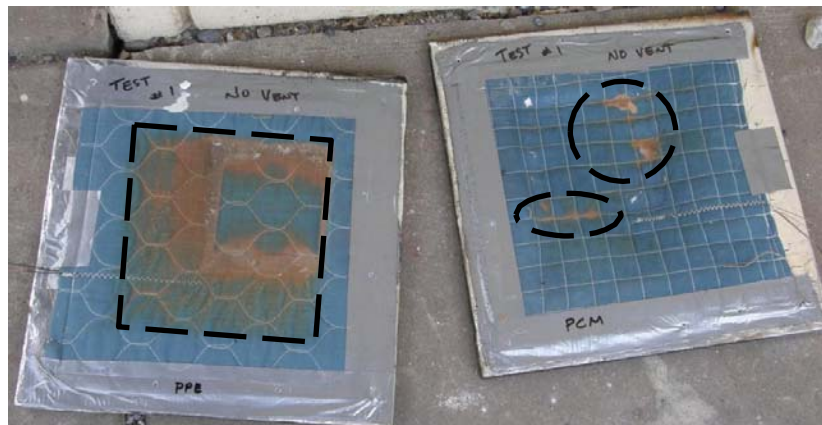
Figure 26: View of the interior liner for the unmodified FFPE assembly (left) and the FFPE assembly with PCM added (right) after Experiment 1. Areas of discoloration highlighted.
