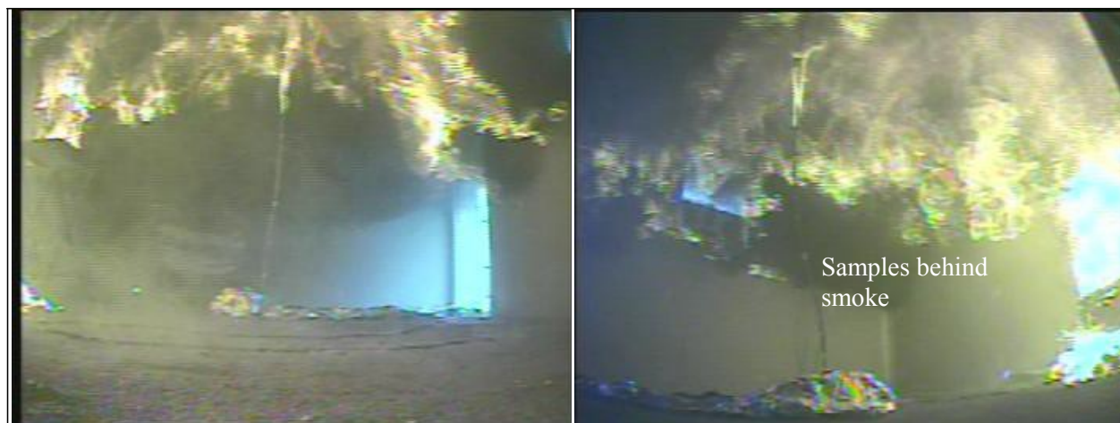
Figure 41: Samples in oxygen-deficient hot layer, above flames, in Experiment 2
