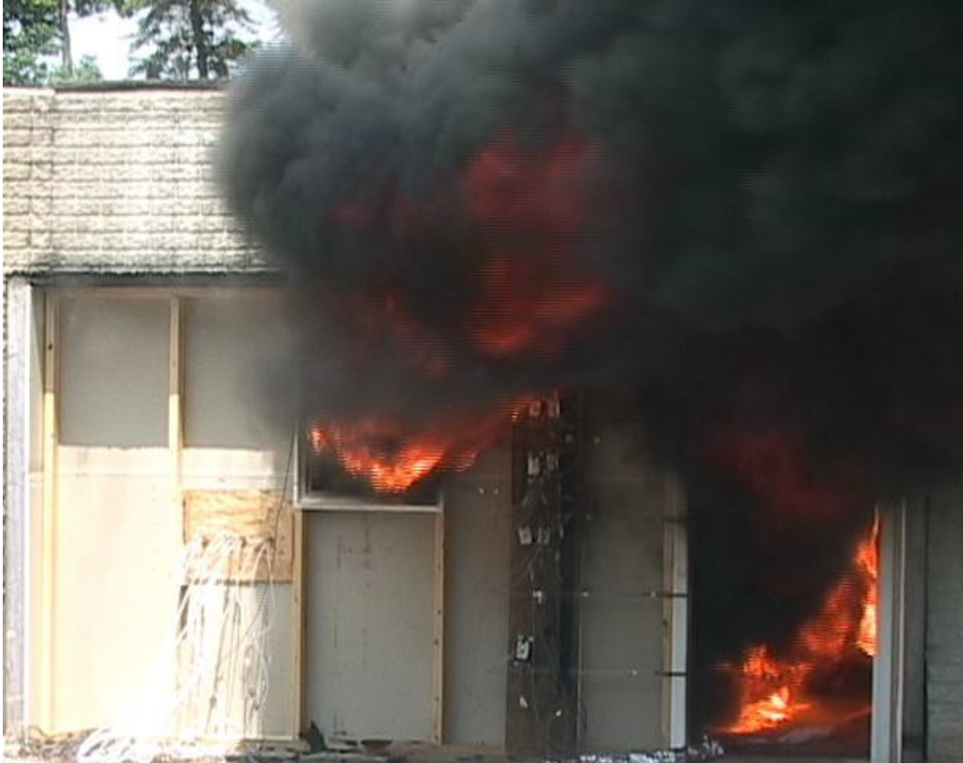
Figure 42: Flames extend from the window and door due to oxygen-depleted (fuel-rich) conditions in the hot gas layer
