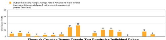
Figure 6: Crossing Ramps Terrain Test Results for Individual Robots
