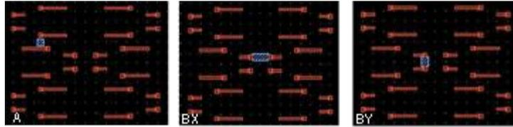
Figure 3. Schematics of an island (“A”) and two bridge (“Bx,” “By”) defects found on 22 nm node SEMATECH Intentional Defect Array (IDA) wafers.
