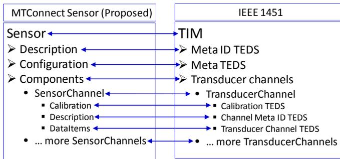
Figure 5 - Mapping between MTConnect and IEEE 1451
