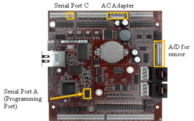
Figure 8 - Hardware setup for IEEE 1451.2 TIM
