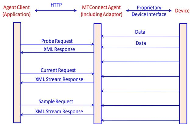
Figure 3 - MTCConnect Communication Protocol
