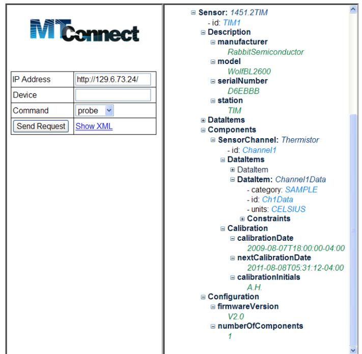
Figure 11 - Screenshot of a Probe request of a MTConnect Agent Client
