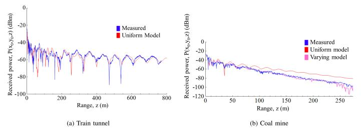
Fig. 5. Experimental results at center frequency  $f_0 = 915$  MHz. In the train tunnel with uniform cross section, the uniform model reliably tracks the measured received power; however, in the coal mine with varying cross section, it falters while the varying model performs well.
