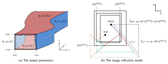
Fig. 2. The varying cross section model. The positive / negative walls may have different electromagnetic properties and their profiles may be asymmetric about the respective axes. The cross section varies throughout the shaft of the tunnel.
