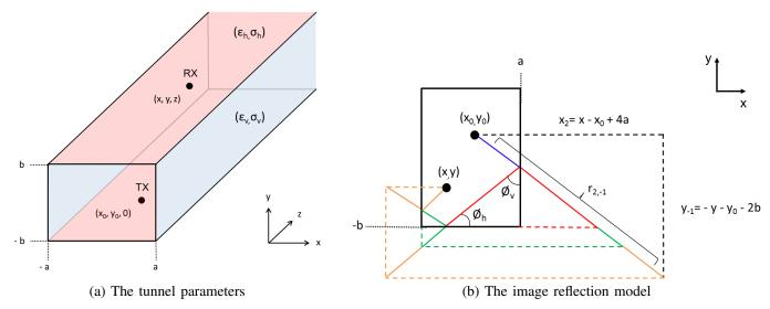
Fig. 1. The uniform cross section model. The vertical and horizontal walls have different electromagnetic properties and their profiles are symmetric about the respective axes. The cross section is uniform throughout the shaft of the tunnel.
