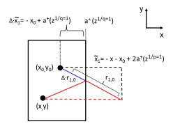
Fig. 3. The reflection point  $z^{1|q=1}$  for (p = 0, q = 1). The marginal distance  $\Delta \cdot r_{1,0}$  traveled from the transmitter to the reflection point can be expressed as a fraction  $\Delta$  of the total distance  $r_{1,0}$  traveled to the receiver.
