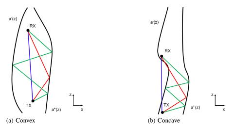
Fig. 4. Positive / negative vertical profiles in the (x, z)-plane. When the profiles are convex, the direct path and all the reflected paths are detected by the receiver, however, when the profiles are concave, they may interfere with some walls.
