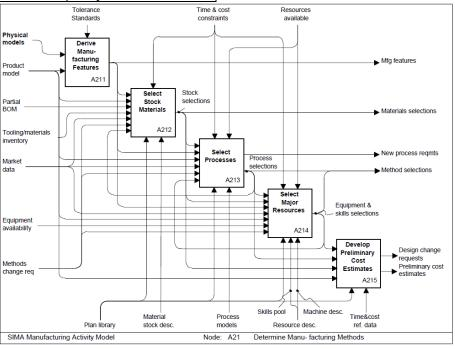
Figure 2 SIMA model: A21 Activity Model- Determine manufacturing methods
