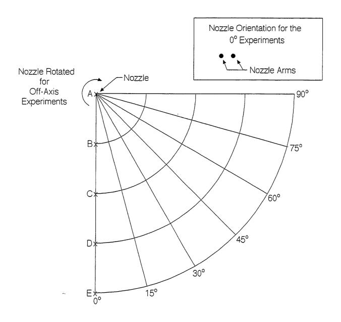
Figure C-3. Plan view of the measurement locations.
