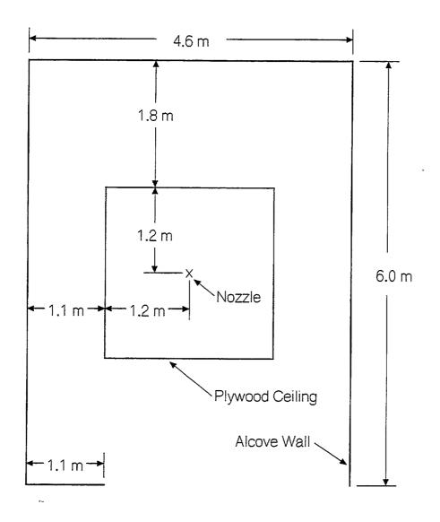
Figure C-1. Plan view of the nozzle alcove.
