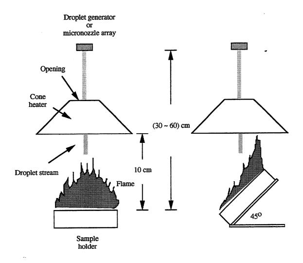
Figure 4. Sample-nozzle configuration.
