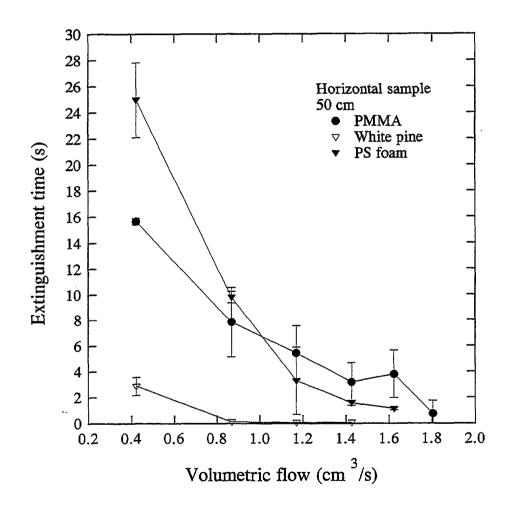
Figure 7. Average extinguishment time as a function of volumetric water flow. The glass nozzle was located at 50 cm above the sample surface.
