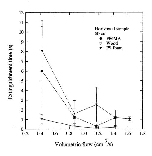
Figure 8. Average extinguishment time as a function of volumetric water flow. The glass nozzle was located at 60 cm above the sample surface.
