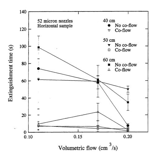
Figure 6. Average extinguishment time as a function of volumetric water flow for PMMA with and without nitrogen co-flow. The 52  $\mu$ m micronozzle array was located at 40 cm, 50 cm, or 60 cm above the fuel surface.
