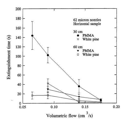
Figure 5. Average extinguishment time versus volumetric water flow for white pine and PMMA. The 62  $\mu$ m micronozzle array was located at 30 cm or 60 cm above the fuel surface.
