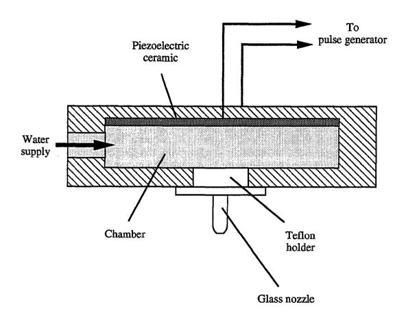
Figure 3. Schematic of the piezoelectric droplet generator.
