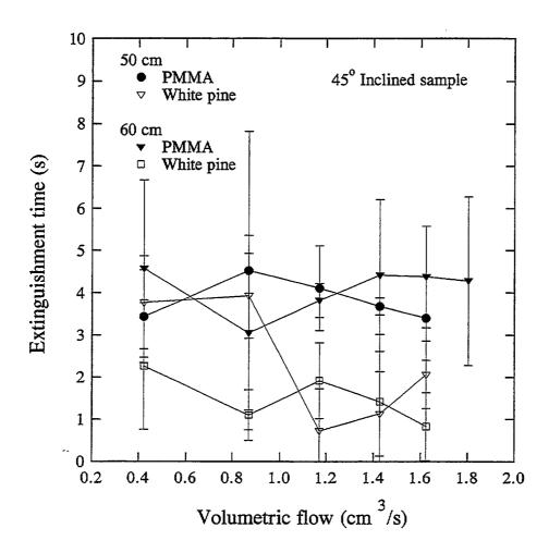
Figure 9. Average extinguishment time as a function of volumetric water flow. The glass nozzle was located at 50 cm or 60 cm above the sample surface. The sample was inclined at 45° with respect to the droplet stream.
