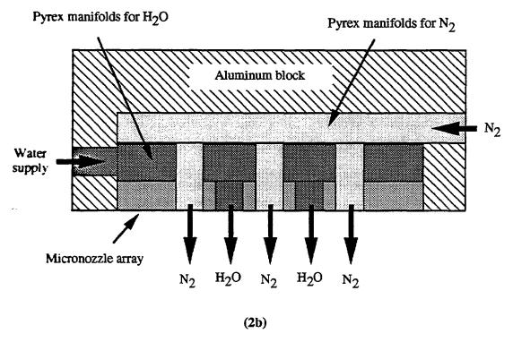
Figure 2. Schematic of micronozzle array.
