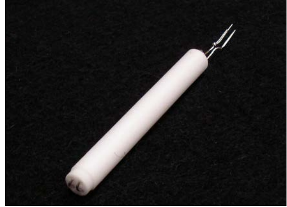
FIGURE 1. A completed resistor assembly from a 22 cm length of wire in a four-bore alumina tube.
