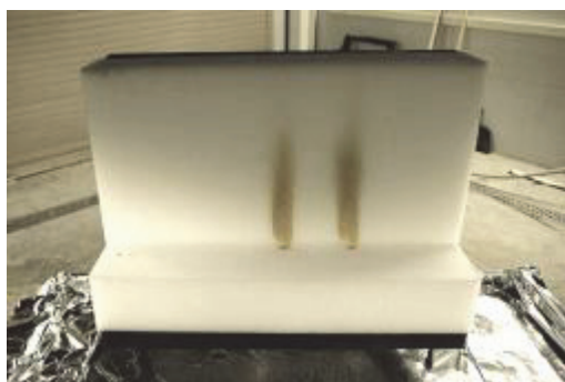
Figure 61. Ignition was not observed after the first 5 s of flame impingement with formulations B5 and C2; a second attempt was carried out by applying the open-flame for other 5 s in a new location 5 in. apart from the original ignition point. Here, it is shown a mockup assembly for formulation C2 after attempting ignition twice.
