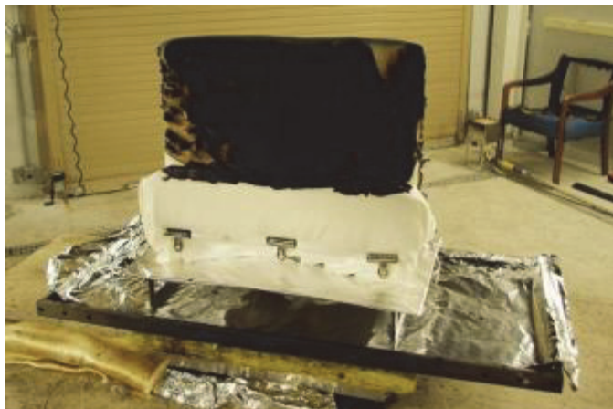
Figure 64. Photo of the residue of the mockup after the open-flame test with barrier material.
