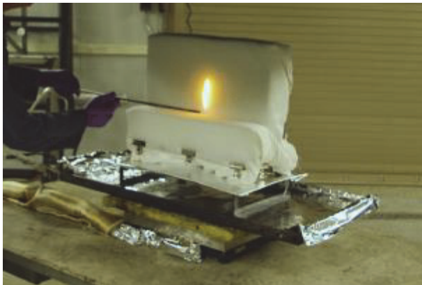
Figure 13. A photo of the 240 mm butane flame impinging on the standard rayon material covering the foam for 70 s in the open-flame test with barrier material.
