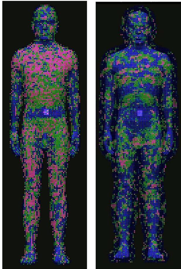
Figure 10. Visualization of Creeping Waves: Left: 0-1 cm distance from body surface; Right: 3-4 cm from body surface
