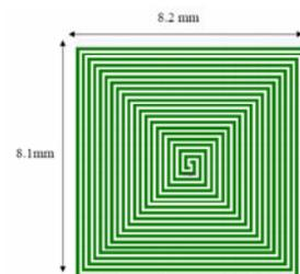
Figure 5. Front view of the implant antenna
