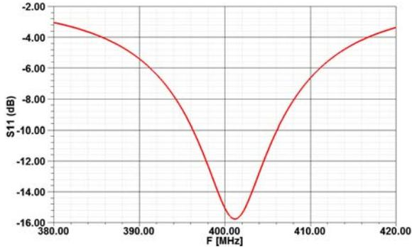
Figure 6. Implant antenna (Return Loss)
