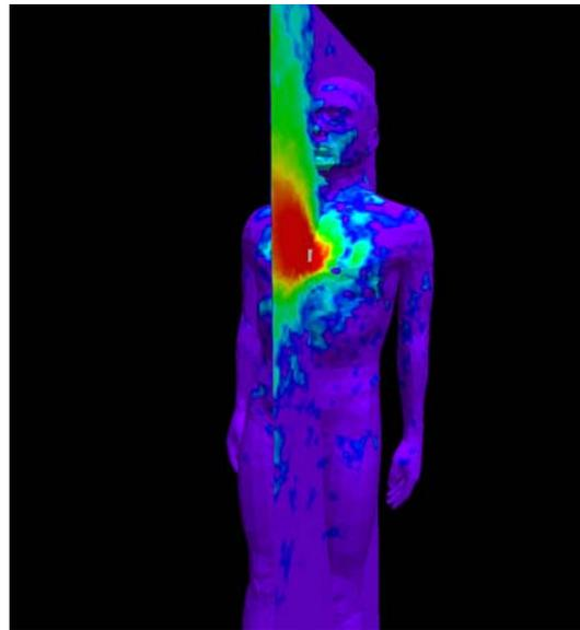
Figure 8. Vertical view of off-body and on-body signal intensity
