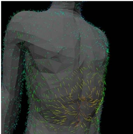
Figure 9. Poynting vector direction on the body surface
