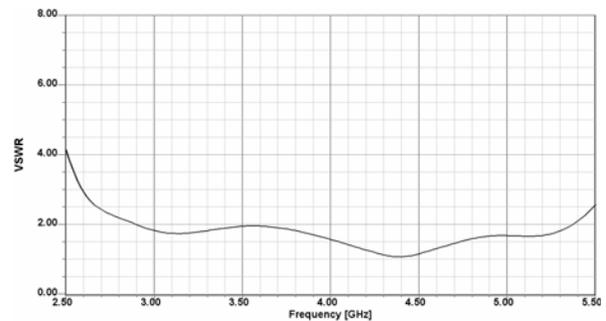
Figure 4. Antenna VSWR on the body surface
