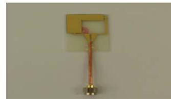
Figure 3. The UWB Antenna
