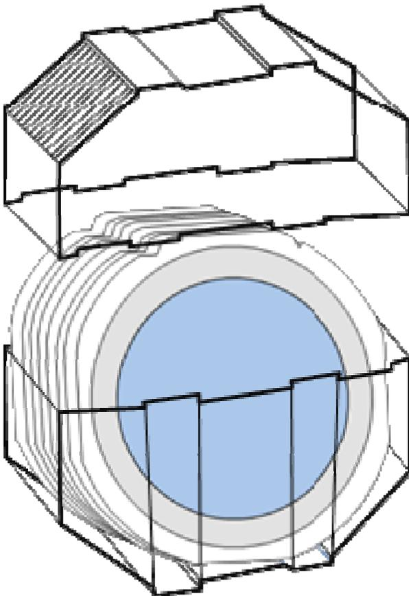
**Figure 5.** Vertical multiple wafer shipping box
