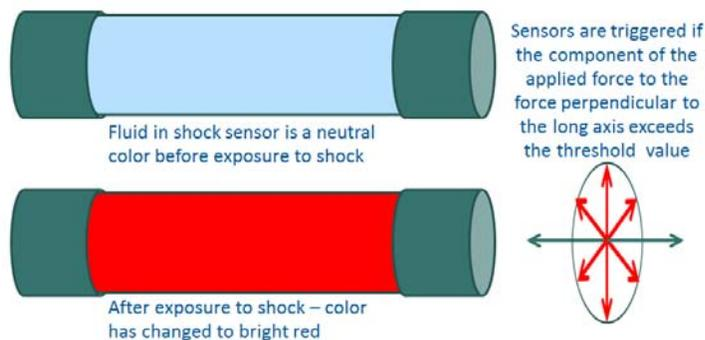
**Figure 7.** Diagram of function of shock sensor
