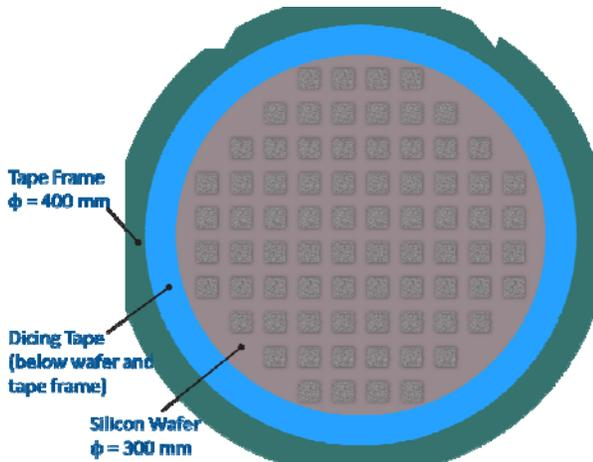
**Figure 1.** 300 mm wafer mounted on tape frame using dicing tape. The tape frame is a 400 mm diameter ring with flats and notches. The locations and dimensions of these feature are defined exactly in SEMI G74 and G87 and enable automated handling. The dicing tape is first attached to the back surface of the tape frame with the adhesive side of the tape facing the front. The wafer is subsequently attached to the adhesive side of the tape.
