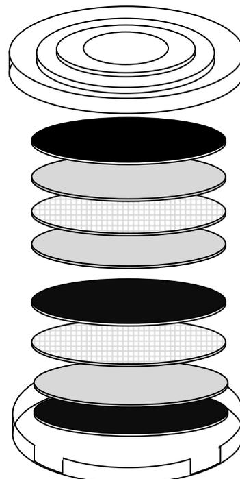
**Figure 2.** Horizontal coin-stack multiple wafer shipping box
