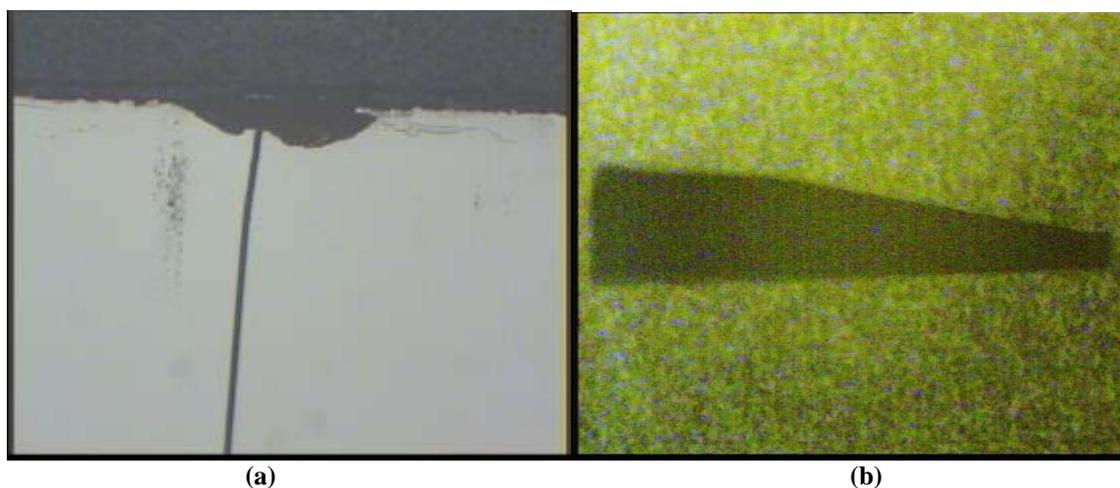
**Figure 8.** Break example from Lot 1, extending from a region of poor edge quality (left) and a break on a Lot 2b wafer, where the force delivered to the wafer was enough to detach a triangular piece of the wafer from the dicing tape (right).
