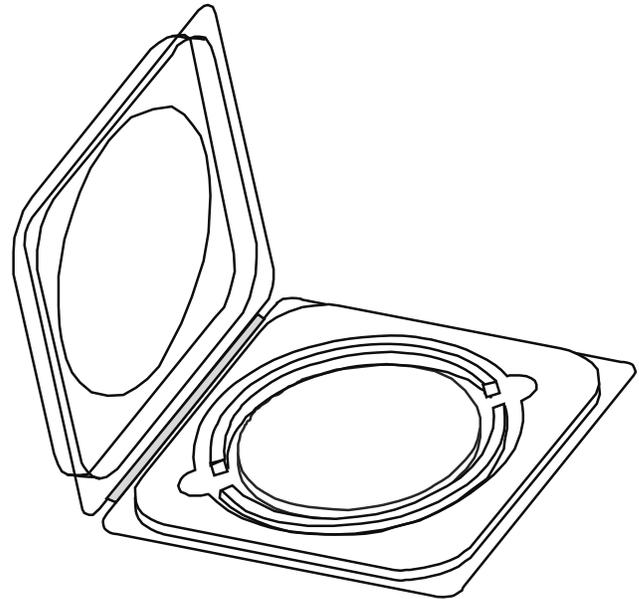
**Figure 4.** Horizontal clamshell stackable shipping box
