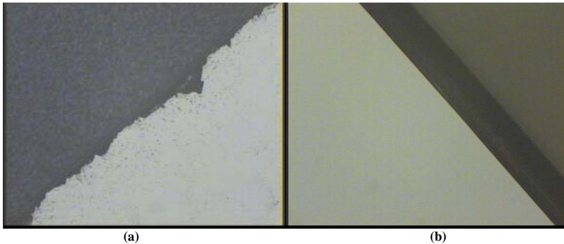
**Figure 6.** Edge quality of typical wafer from Lot 1 (a) and Lot 2b (b) after debonding.
