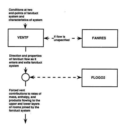
Figure 3.4.6. Use of the algorithms VENTF, FANRES, and FLOGO2 to carry out rates of exchange of mass, enthalpy, oxygen, and other products of combustion through fan/duct forced ventilation systems connecting two rooms of a multiroom facility.
