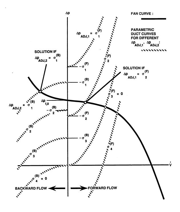
Figure 3.4.4. Graphical presentation of the problem of solving Eq. (3.4.24) and finding the direction and flow rate through a fan/duct system.
