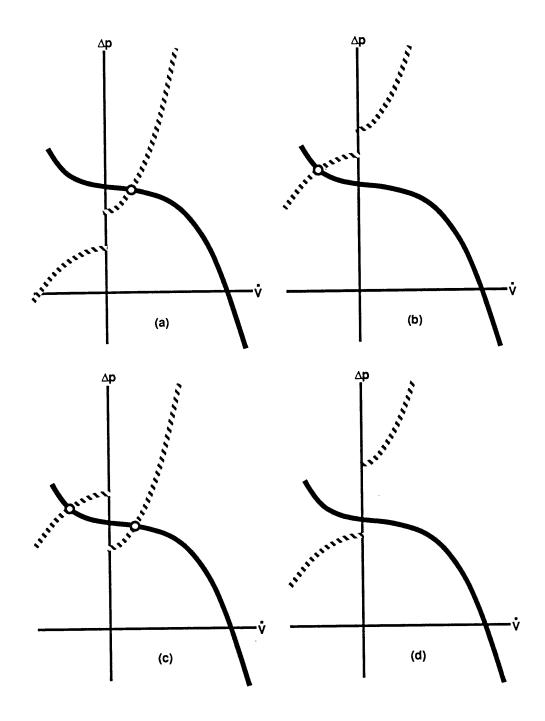
Figure 3.4.5. Graphical presentation from Figure 3.4.4 of the four classes of solution for flow rate through the fan/duct system: (a) single forward-flow solution and no backward-flow solution, (b) single backward-flow solution and no forward-flow solution, (c) one forward-flow solution and one backward-flow solution, and (d) no solutions.
