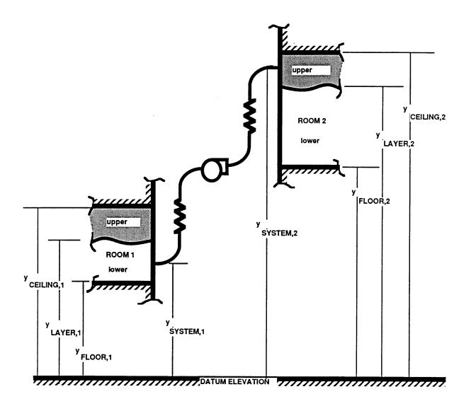
Figure 3.4.1. The fire-generated environment in two rooms connected by a fan/duct system.
