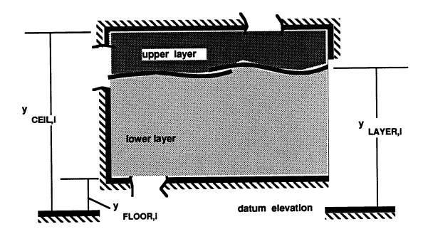
Figure 2.1. The two-layer environment for an arbitrary room of a multi-room facility.
