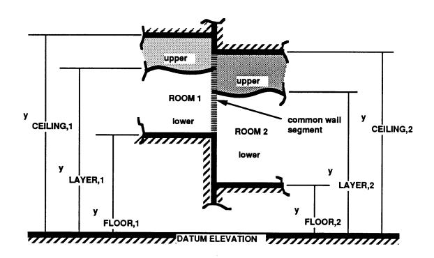
Figure 3.3.1. The fire-generated environment in two adjacent rooms.
