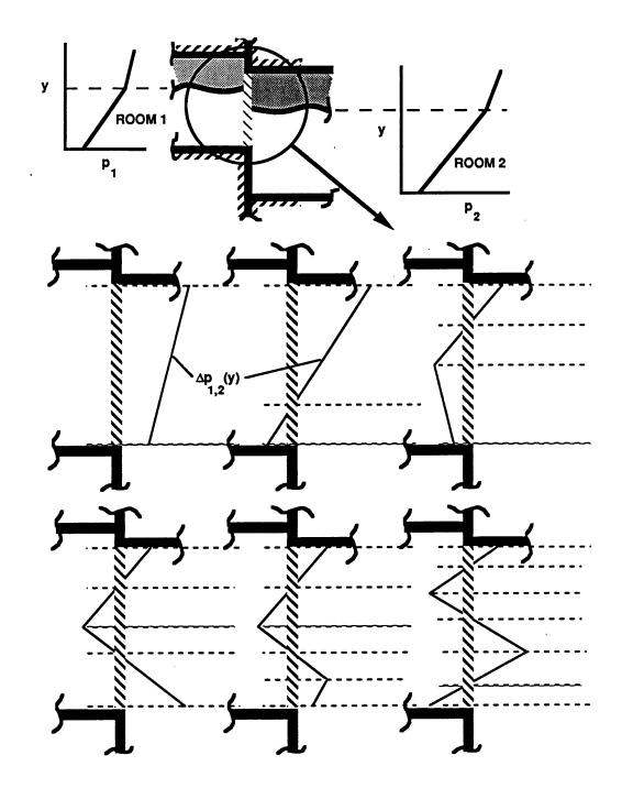
Figure 3.3.2. Possible distributions of  $\Delta p_{1,2} = p_1 - p_2$  for a common-wall segment.
