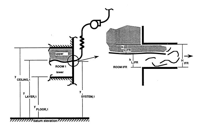
Figure 3.4.3. An illustration of the flow entering the duct in room iFR when the layer interface is between the top and bottom of the vent opening.
