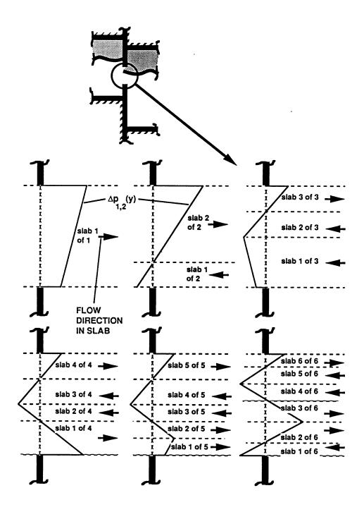
Figure 3.3.3. Possible distributions of  $\Delta p_{1,2} = p_1 - p_2$  for a single vent and the flow directions of its uniform-property flow slabs.
