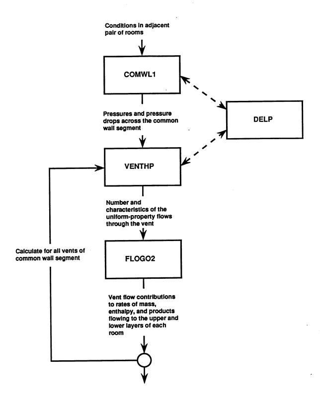
Figure 3.3.4. Use of the algorithms DELP, COMWL1, VENTHP, and FLOGO2 to carry out rates of exchange of mass, enthalpy, oxygen, and other products of combustion through vertical natural vents of a multi-room facility.
