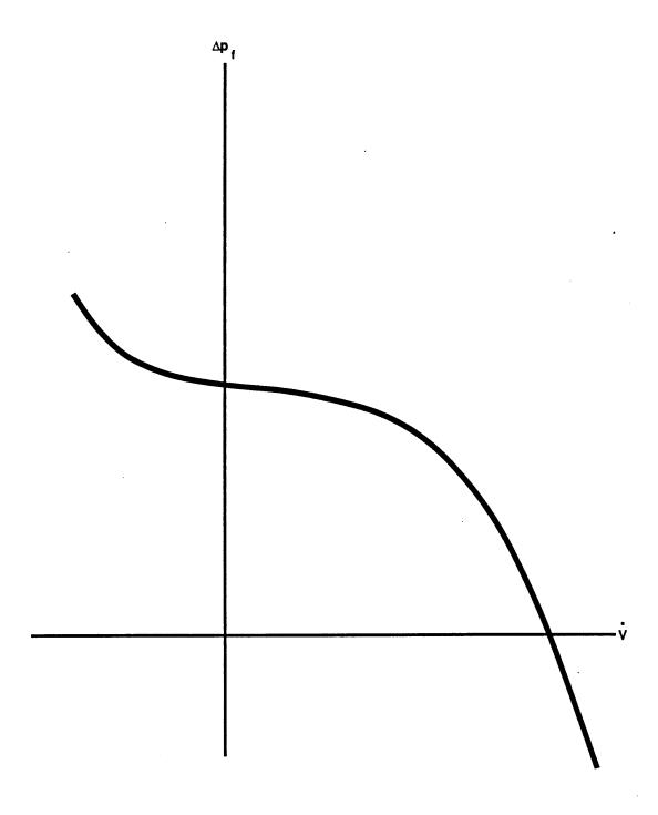
Figure 3.4.2. A sketch of a generic fan operating curve which increases monotonically in volume flow rate with decreasing cross-fan pressure difference.
