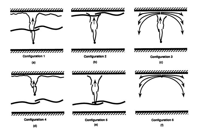
Figure 3.2.2. Configurations for the fire, the plume and the elevations of interface and ceiling.
