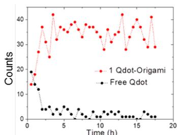
**Fig. 2** Binding reaction of Qdots to DNA origami containing a single binding site. The counts (number observed in 30 min increments) of free Qdot decreases as the reaction progresses, while the counts of Qdot-Origami increases. Free and bound Qdots are easily identified by their different diffusion coefficients.
