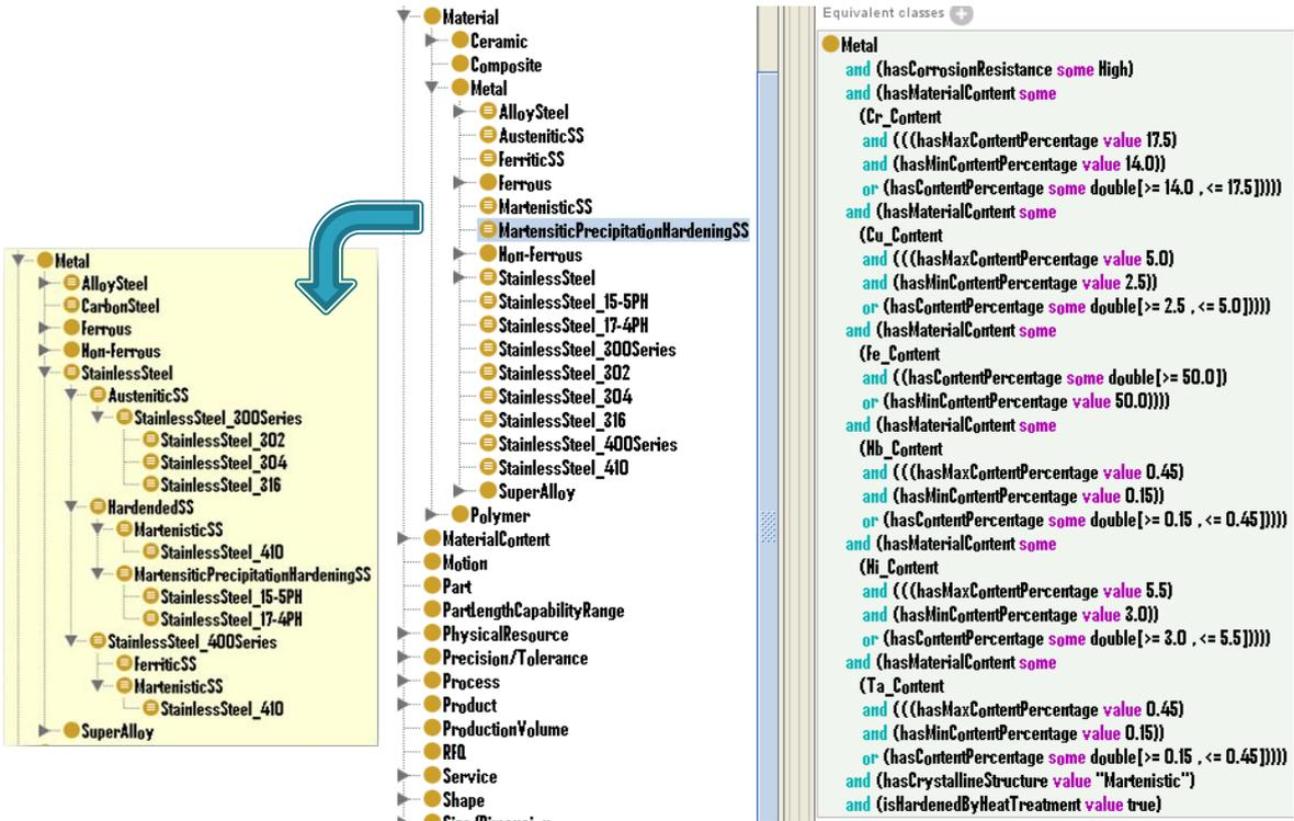
Fig. 5. Definition of *Martensitic precipitation hardening stainless steel*
