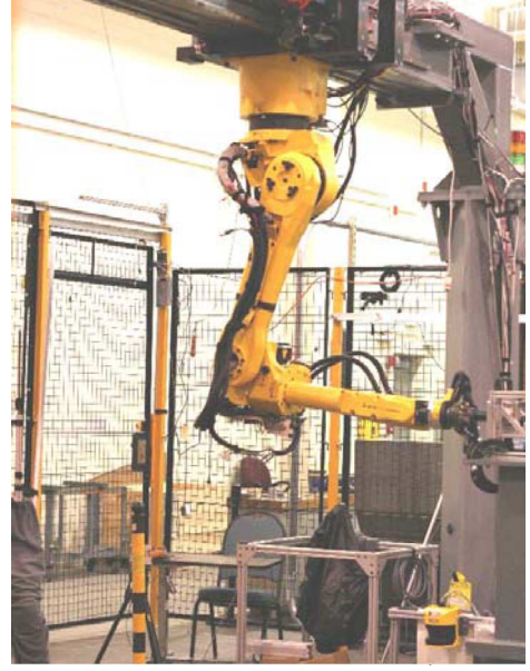
Fig. 2. The inverted 6DOF robot arm mounted on a 7th axis rail. The workcell is monitored by dual safety laser scanners (one shown in the lower-right) and protected by a fence with three gate interlocks (one shown on the left).
