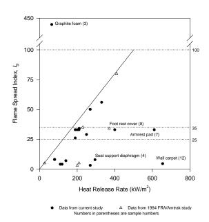
Figure 1. Comparison of  $I_s$  as measured according to ASTM E 162 / D 3675 and peak HRR as measured in the Cone Calorimeter.
