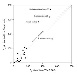
Figure 4. Comparison of ASTM E 662  $D_s$  (4.0) with calculated Cone Calorimeter  $D_s$  (1.0)
