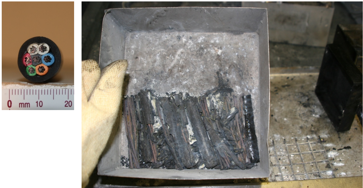
Figure 4-9. Cross section of Cable 802 and photograph of burn residue.
