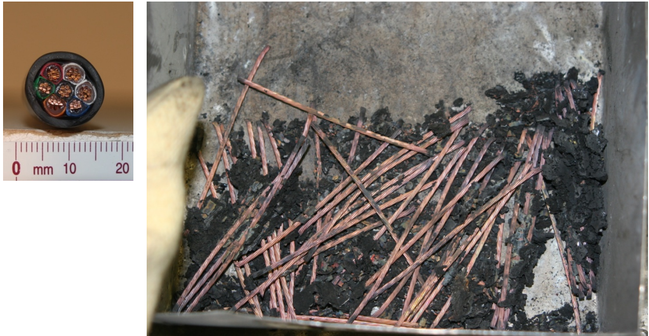
Figure 4-19. Cross section of Cable 807 and photograph of burn residue.
