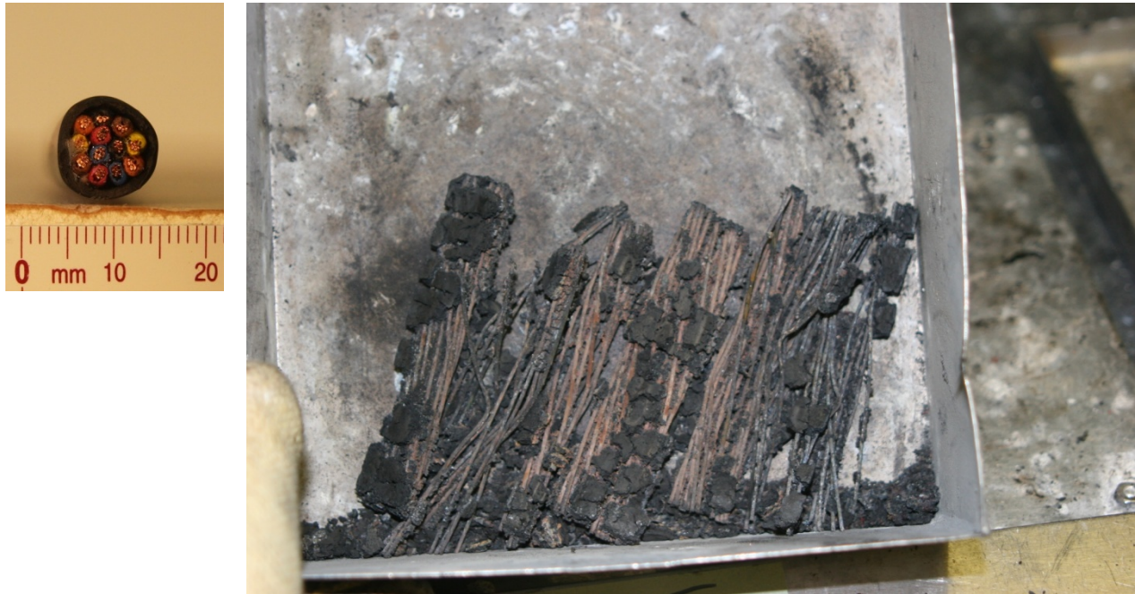
Figure 4-35. Cross section of Cable 815 and photograph of burn residue.
