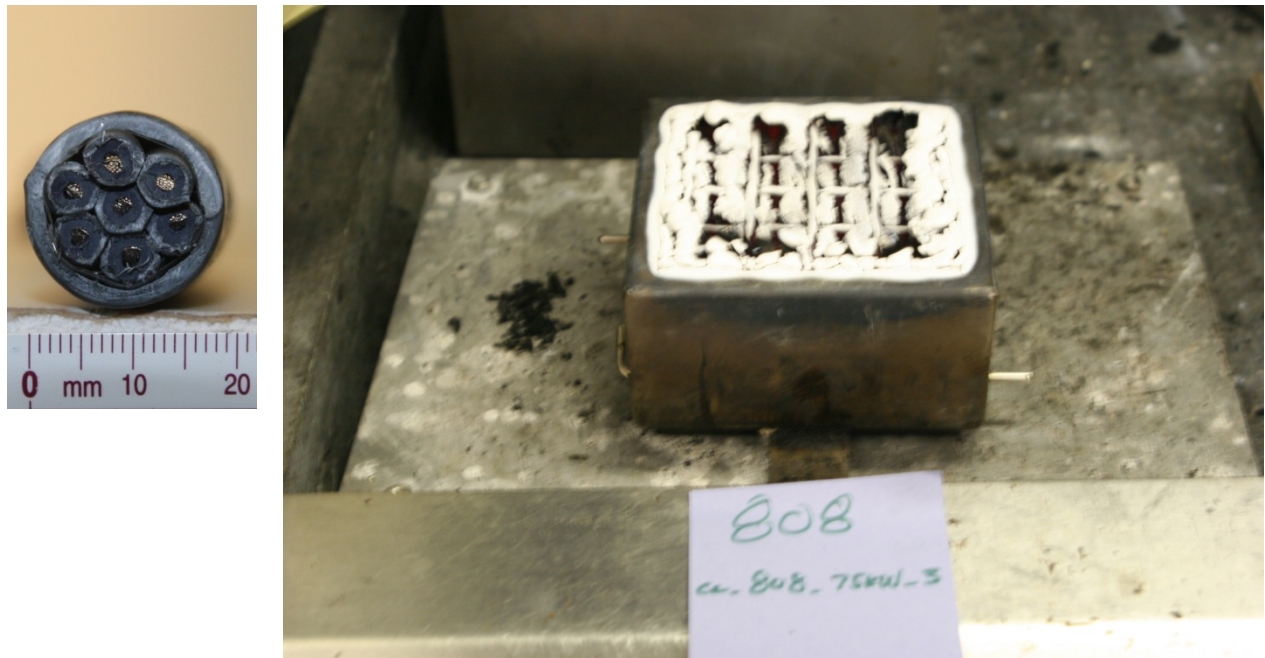
Figure 4-21. Cross section of Cable 808 and photograph of burn residue.
