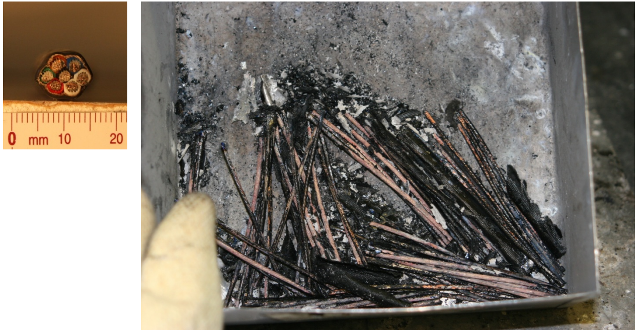
Figure 4-15. Cross section of Cable 805 and photograph of burn residue.
