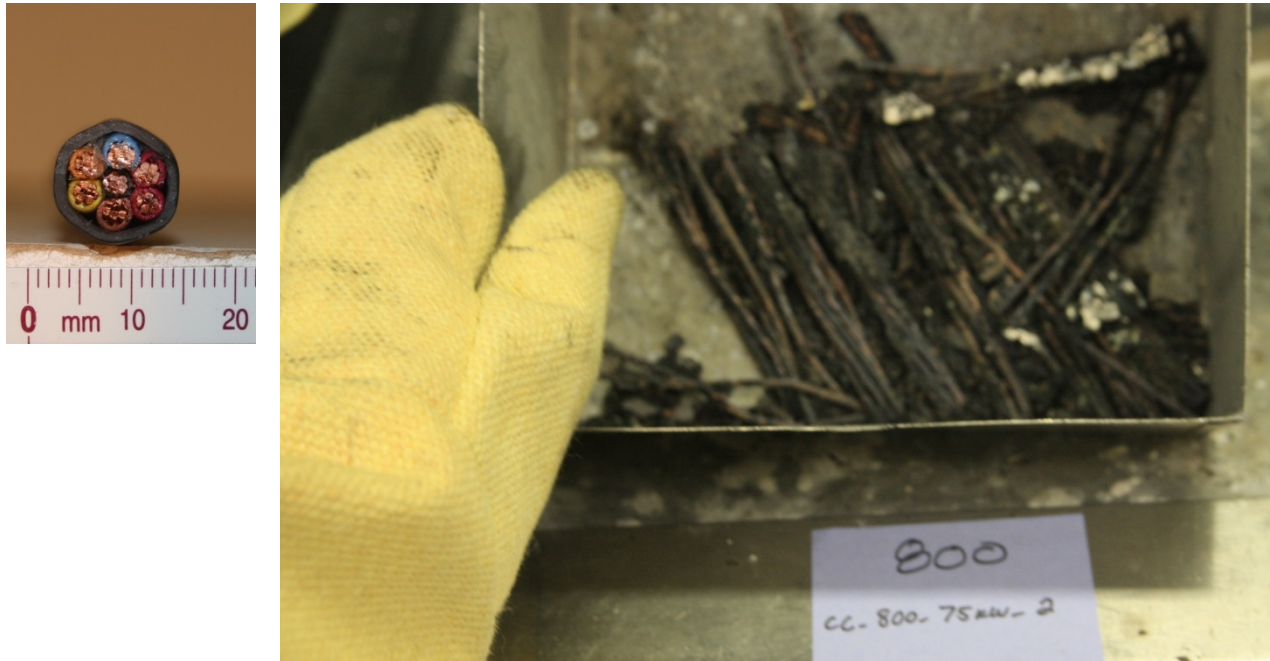
Figure 4-5. Cross section of Cable 800 and photograph of burn residue.
