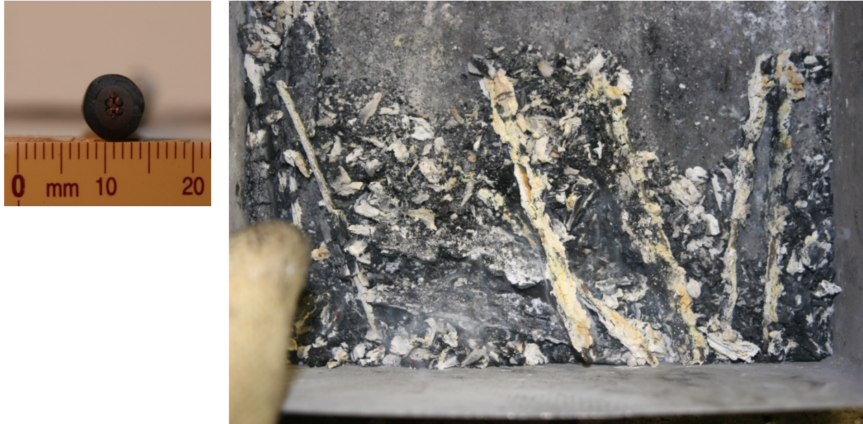
Figure 4-50. Cross section of Cable 824 and photograph of burn residue.
