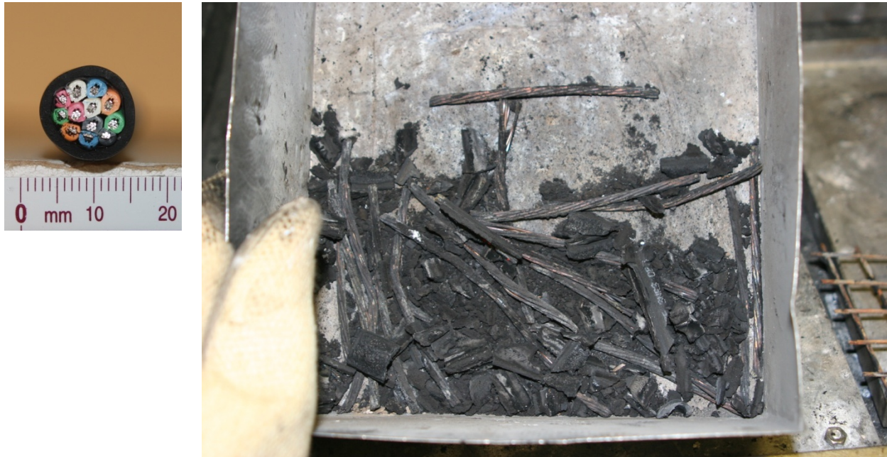
Figure 4-31. Cross section of Cable 813 and photograph of burn residue.
