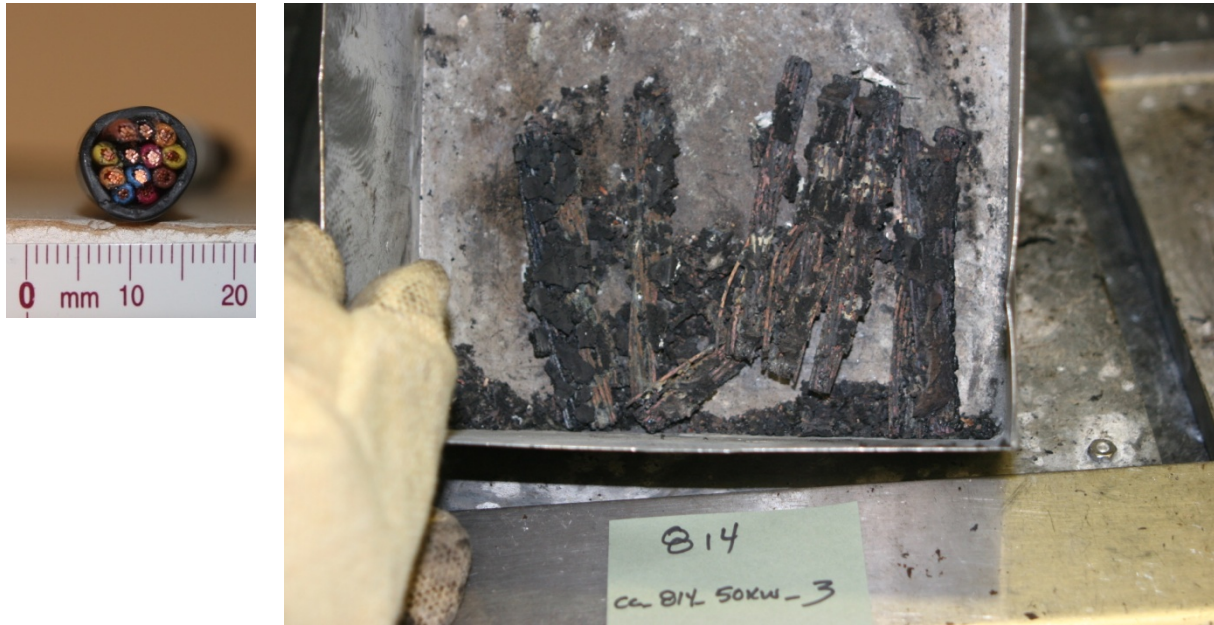
Figure 4-33. Cross section of Cable 814 and photograph of burn residue.
