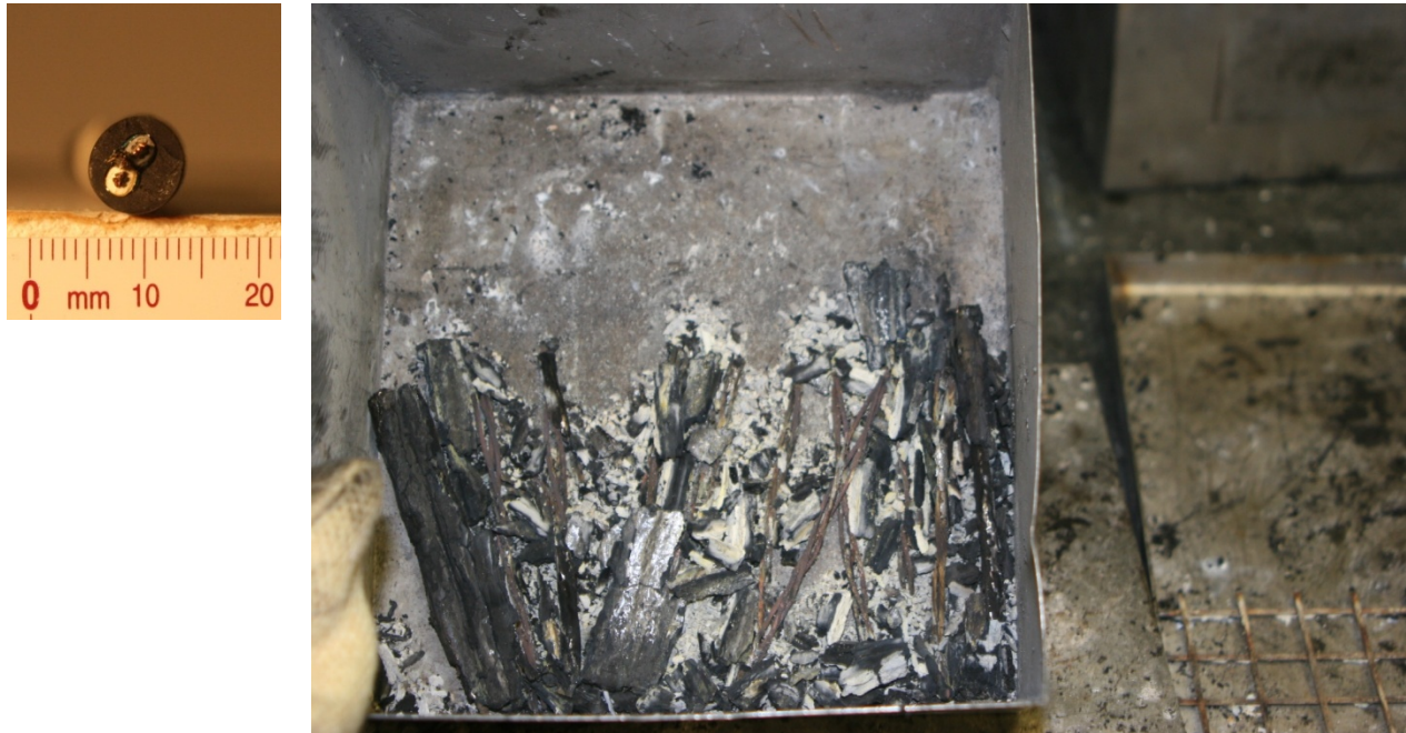
Figure 4-39. Cross section of Cable 817 and photograph of burn residue.
