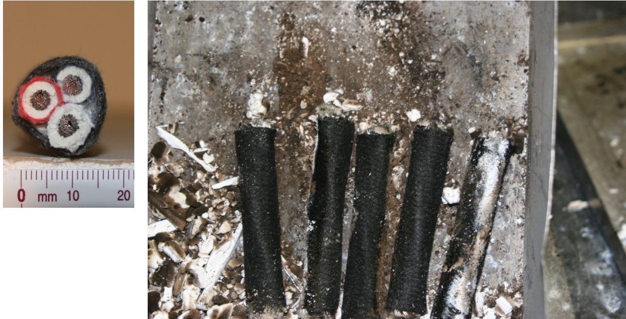
Figure 4-43. Cross section of Cable 819 and photograph of burn residue.
