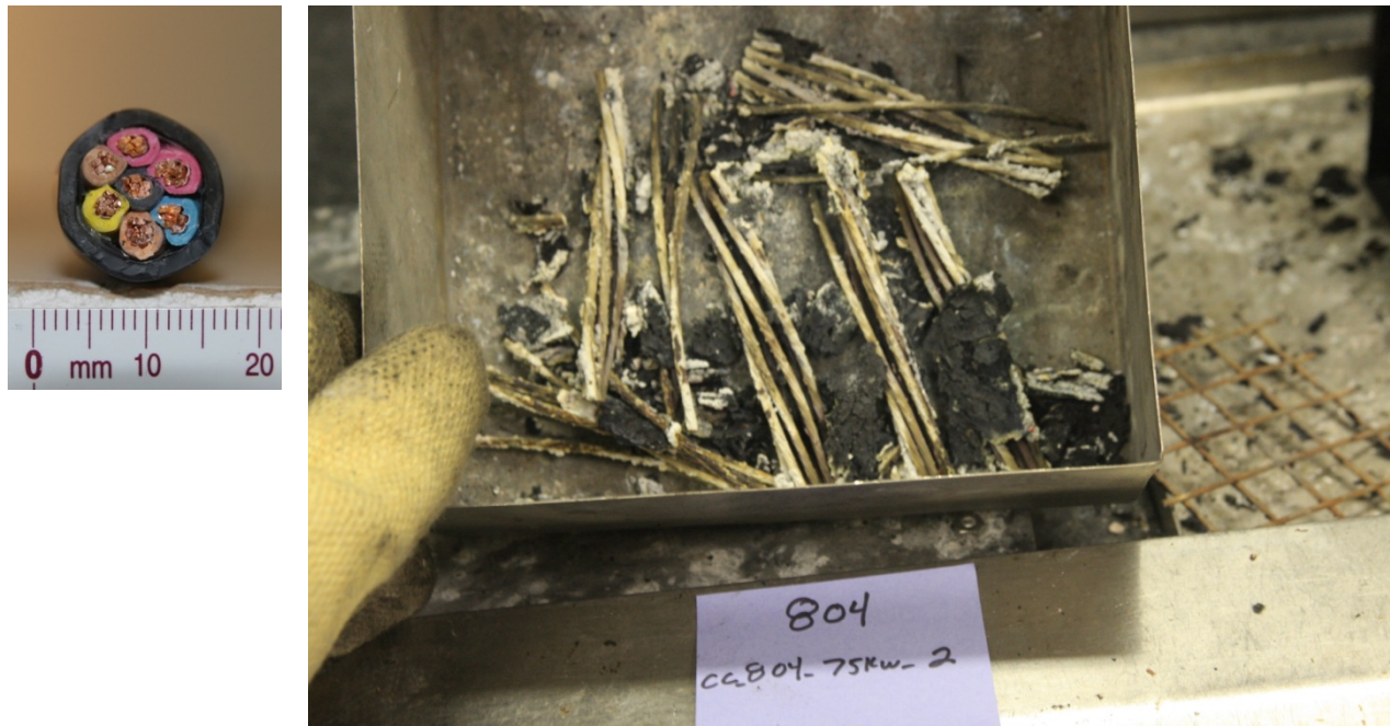
Figure 4-13. Cross section of Cable 804 and photograph of burn residue.
