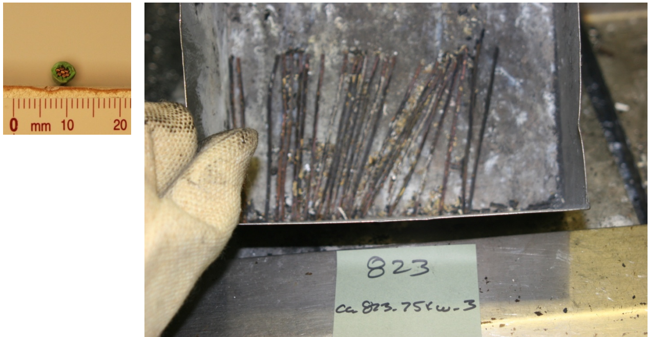
Figure 4-48. Cross section of Cable 823 and photograph of burn residue.
