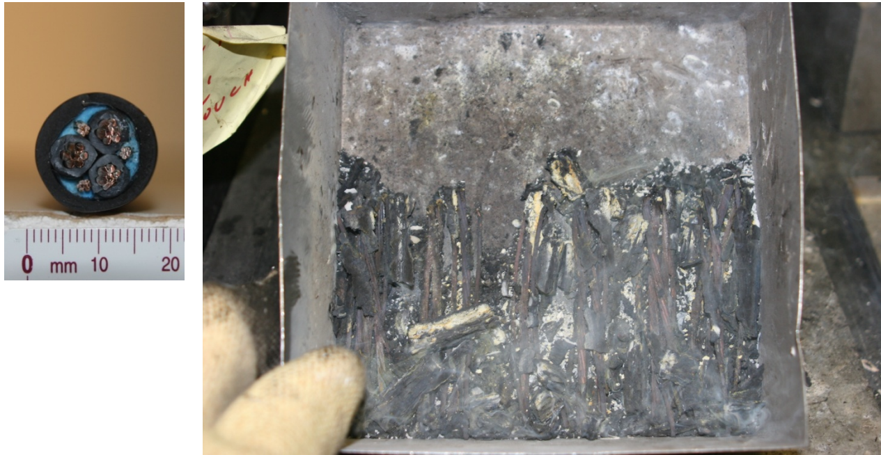
Figure 4-29. Cross section of Cable 812 and photograph of burn residue.
