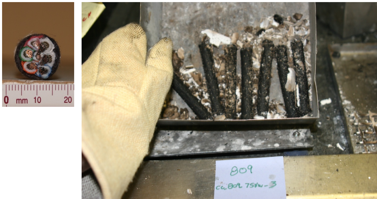
Figure 4-23. Cross section of Cable 809 and photograph of burn residue.
