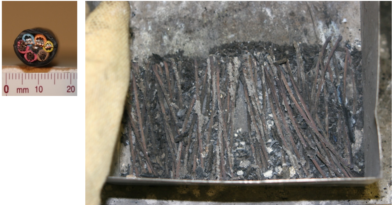
Figure 4-17. Cross section of Cable 806 and photograph of burn residue.
