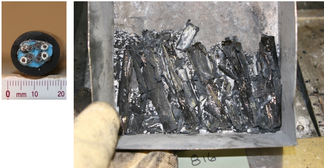
Figure 4-37. Cross section of Cable 816 and photograph of burn residue.
