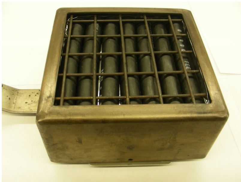
Figure 4-3. The completed specimen assembly for the cone calorimeter.
