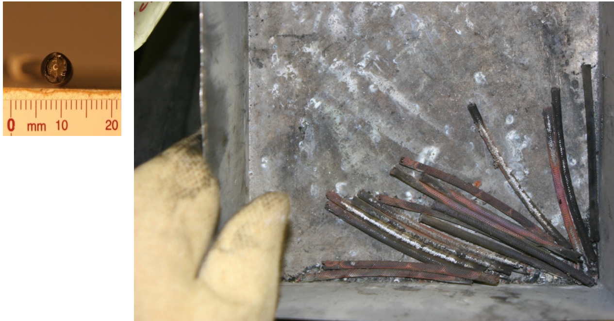
Figure 4-41. Cross section of Cable 818 and photograph of burn residue.
