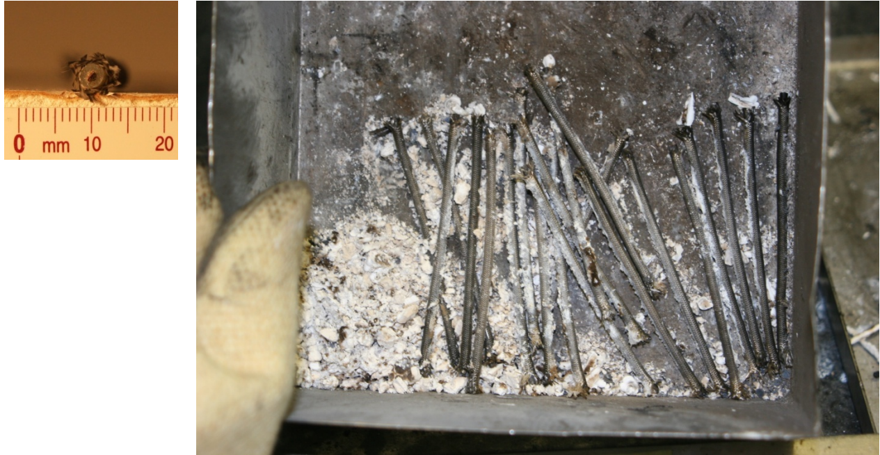
Figure 4-46. Cross section of Cable 822 and photograph of burn residue.
