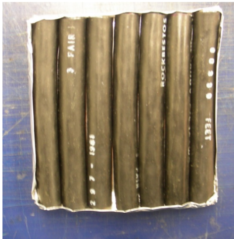
Figure 4-1. Typical cable sample for cone calorimeter.
