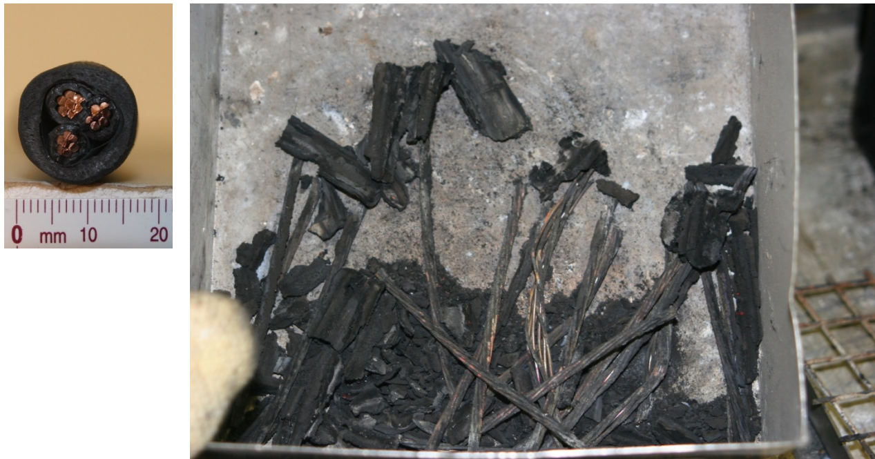
Figure 4-27. Cross section of Cable 811 and photograph of burn residue.
