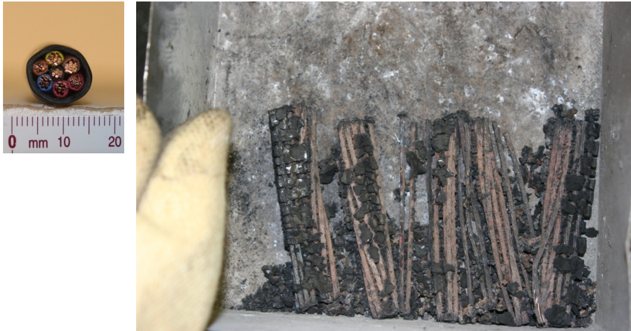
Figure 4-7. Cross section of Cable 801 and photograph of burn residue.
