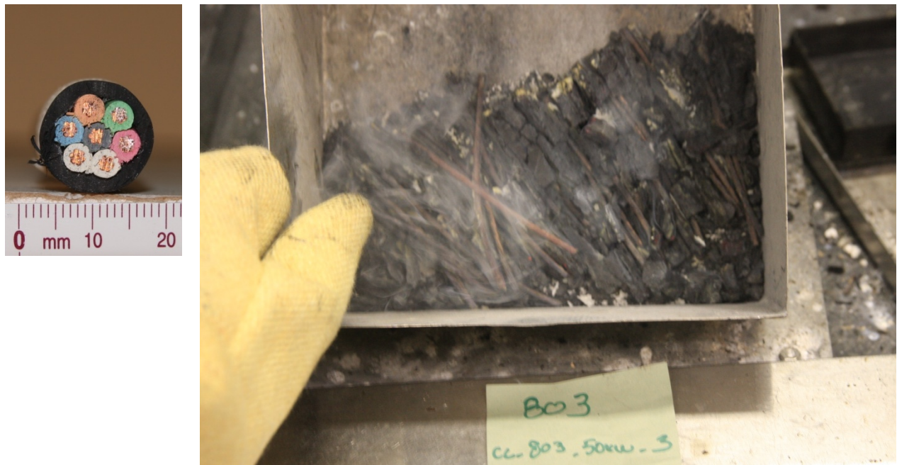
Figure 4-11. Cross section of Cable 803 and photograph of burn residue.
