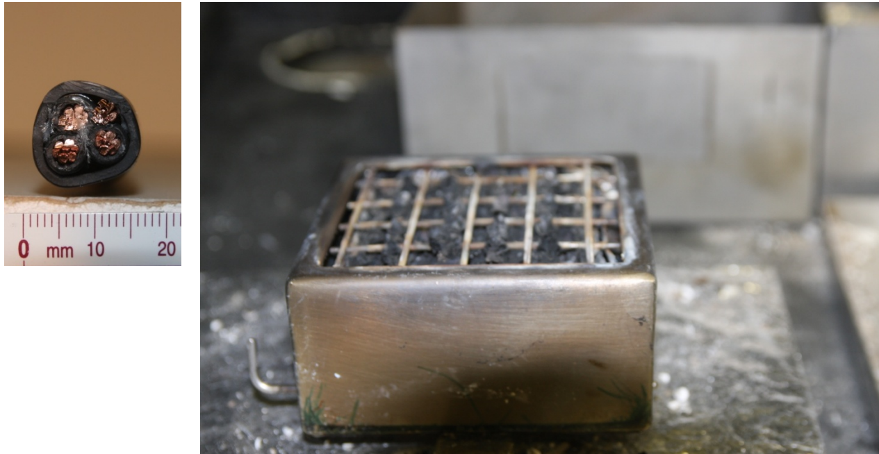
Figure 4-25. Cross section of Cable 810 and photograph of burn residue.
