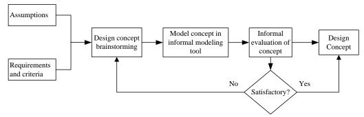
Figure 3: The design concept development process
