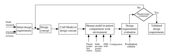
Figure 2: Requirements evaluation process
