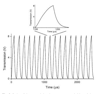
Fig. 3 Series of ring-up and ring-down events recorded in real-time at a given laser frequency. The acquisition rate was  $\approx$ 7 kHz and was limited by the cavity response time itself. The relative standard deviation of the measured ring-down time constants was  $\approx$ 0.008 %
