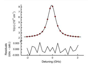
**Fig. 5** Typical measured spectrum and speed-dependent Nelkin-Ghatak [23] fit of the (30012)  $\leftarrow$  (00001) *P*14e CO<sub>2</sub> transition for a sample of CO<sub>2</sub> in air ( $\approx$ 4,400 µmol/mol) at a pressure of 13.3 kPa. The shown spectrum has a signal-to-noise ratio of 3,200:1 and is an average of 6 individual spectra each recorded in  $\approx$ 2.6 ms
