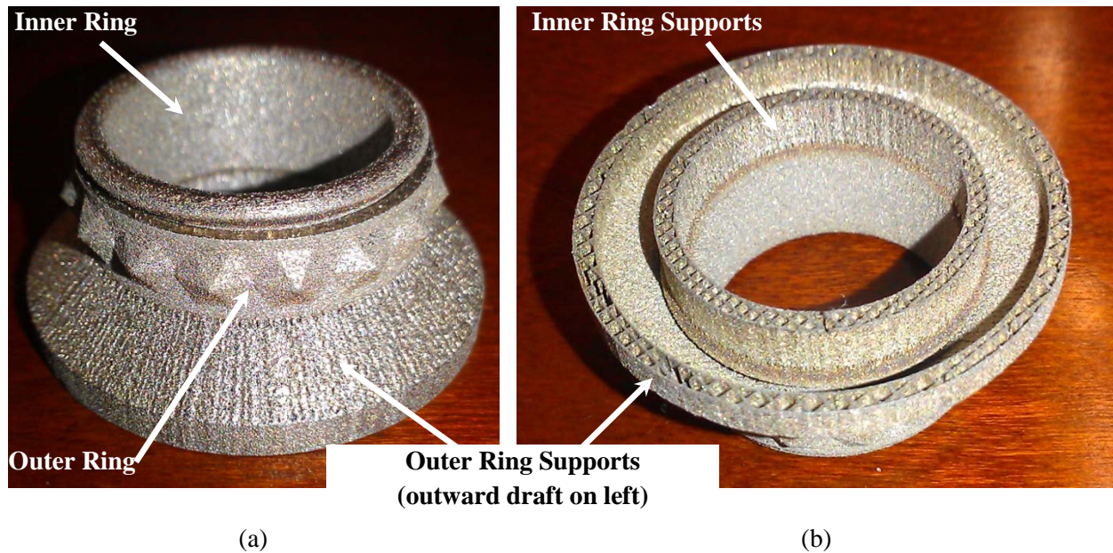
Figure 7: A ring that has an outer section that rotates freely about the inner section: (a) front view, (b) bottom view.
